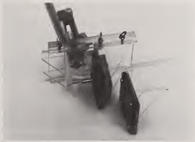
Figure 1. Apparatus for holding tissue specimens which allows accurate determination of region being examined. Ball-ended rod for transducer alignment is shown mounted. A holder for heart valves is on the table. Pointed rod is a transfer marker used only for initial alignment. This apparatus is suspended in a temperature-controlled saline bath for measurements.
