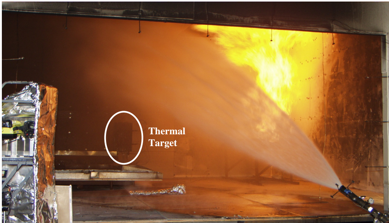
Figure 5—5. Visible image of typical hose stream test set up. Three TIC (behind foil on far left) are viewing a thermal target through a fog spray in the presence of a 2.2 MW heptane fire.
