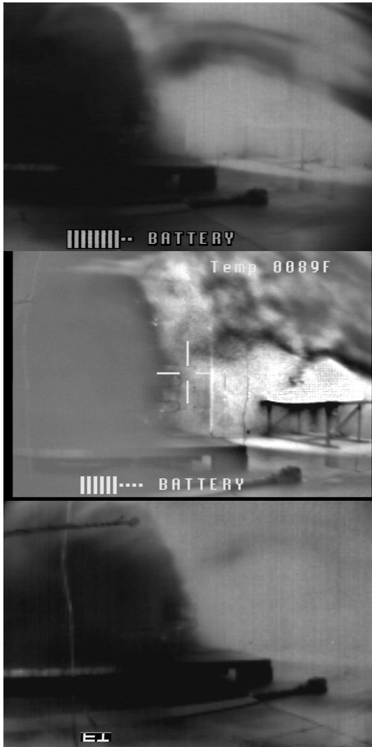
Figure 5—13. Thermal images of a scene in which a fog spray is directed toward a wall in front of a 2.2 MW heptane fire. A BST-type TIC produced the center image and ASi-type TIC from different manufacturers produced the two other images.
