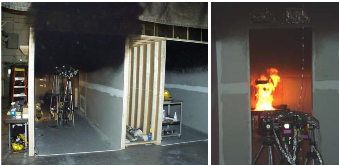
Figure 5—2. TIC are positioned in the hot upper layer viewing a target through heavy toluene smoke, test configuration D (left), and in the lower layer viewing flames and high heat conditions, test configuration A (right).
