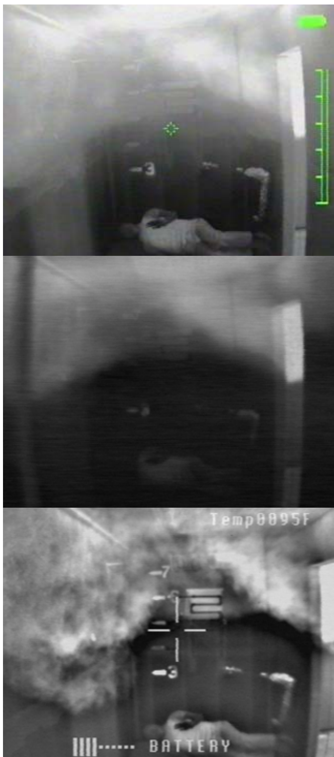
Figure 5—15. Identical scene from full scale test series two observed with three different cameras. From top to bottom VOx, ASi, and BST TIC are utilized to view the same scene at the same time consisting of a mock victim on the floor with smoke and flames in the field of view.
