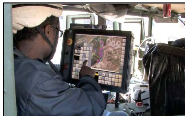
Figure 2. Participant using the 18" vehicle-mounted operator control unit (OCU) within the OCU HMMWV.
