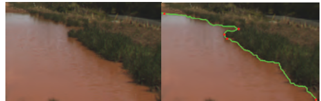
Figure 4. The GIMP image viewer has an intelligent scissors tool to segment image regions along contours. We have extracted the intelligent scissors portion of GIMP and have integrated it into our ground truthing tool. In this example, only 5 vertices were needed along the cropped portion of the water boundary. Intelligent scissors is run for each pair of neighbor vertices to segment the water's edge.
