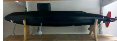
Figure 8: A SCUUL UUV equipped with reflective markers.
