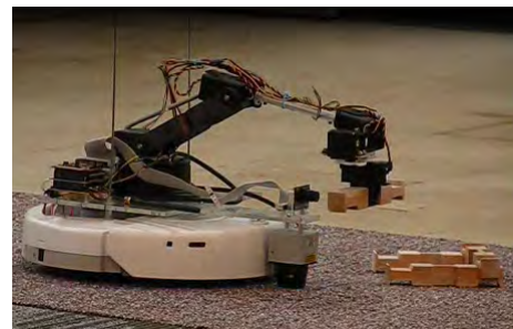
Figure 3: The mini mobile manipulator ( M^3 ) robot assembled from the iRobot Create and Lynxmotion platform assembling a 2-D structure out of interlocking blocks.
