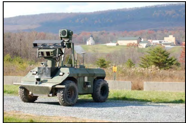
Figure 1. Experimental Unmanned Vehicle (XUV) from the U.S. Army Research Laboratory was used as the UGV in this field assessment.
