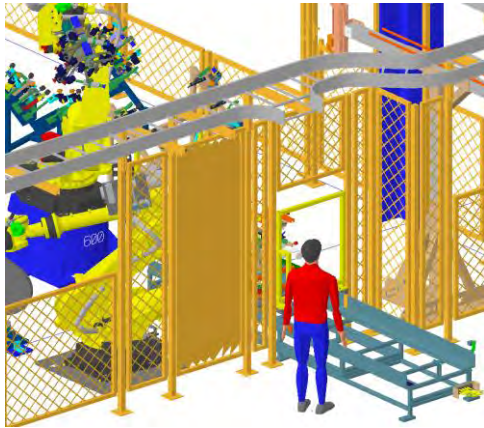
Figure 2 A Workpiece is Transferred out of Robot Workcell in order for the Human to Perform an Inspection Task
