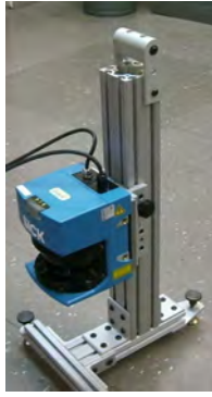
Figure 1: Adjustable and portable apparatus for mounting the LMS
