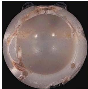
Worn UHMWPE cup of total hip replacement.
