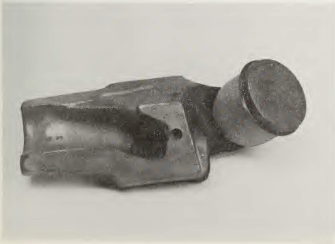
Figure 9 Head Section Of Figure 1 With Cup Packed, Ready For Boronizing.
