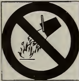
Do Not Use Water To Extinguish (Black on White, Red Circle & Slash)
