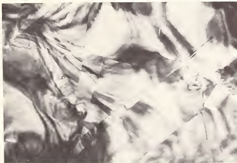
Fig. 8. Characteristic zig-zag and triangular domains of B-Nd 2 O 3 in crystals of A-Nd 2 O 3 (X 30.000).
