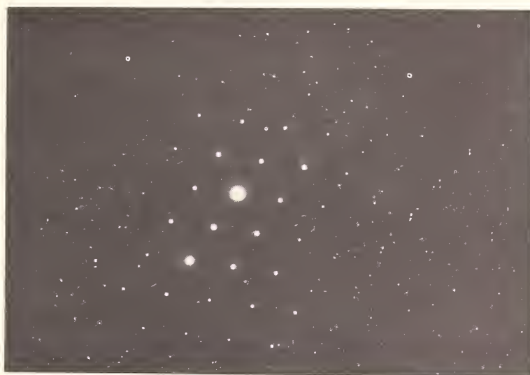
Fig. 5. Electron diffraction of a crystal of monoclinic B-Sm 2 O 3 . The electron beam is along [10 \bar{1} ], 3.5° off the plane of the thin film which is parallel to (201).
