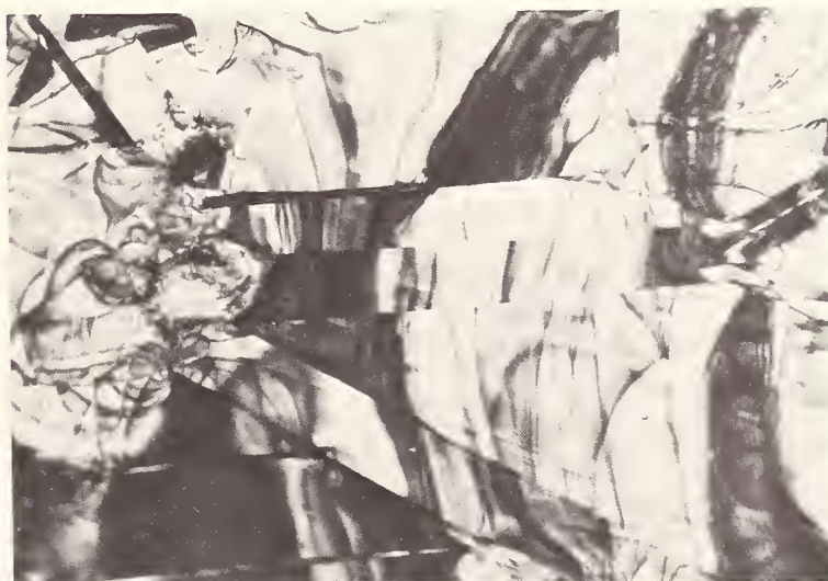
Fig. 9. Twinning and dislocations in B-Sm 2 O 3 . Twins are {313} and {111} (X 30.000).
