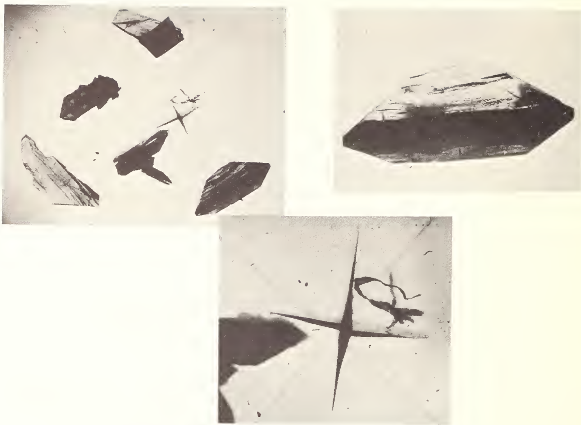
Fig. 5. Photographs of typical twinned crystals of the orthorhombic phase(s) in the \text{Nb}_2\text{O}_5\text{-ZrO}_2 system grown in the \text{BaO}:\text{V}_2\text{O}_5 flux.
