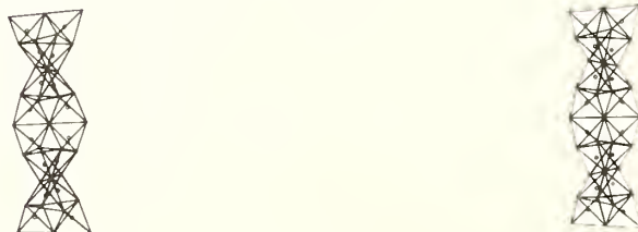
Fig. 6. Stereoscopic view of the infinite column of tetrahedra in \text{Ba}_6\text{Fe}_8\text{S}_{15} . The vertical direction is [001] of the unit cell.
