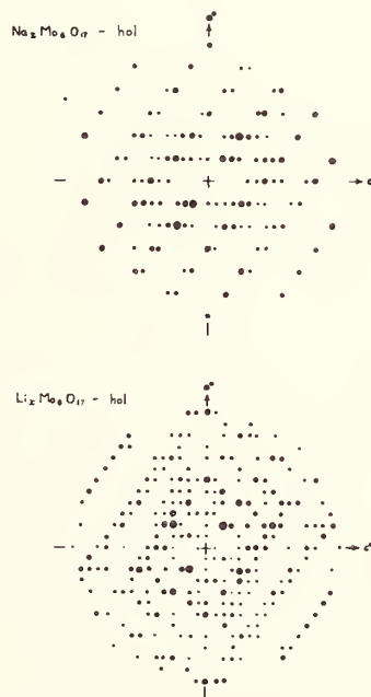
Fig. 4. Intensity weighted reciprocal lattice zero levels for \text{Li}_x\text{Mo}_6\text{O}_{17} and \text{Na}_x\text{Mo}_6\text{O}_{17} .
