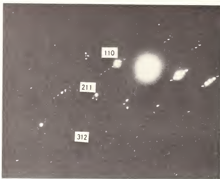
Fig. 7. \text{Cr}_2\text{Ti}_n-2\text{O}_{2n-1} , 12 < n < 22 : superlattice direction lying between [211] and [312] .
