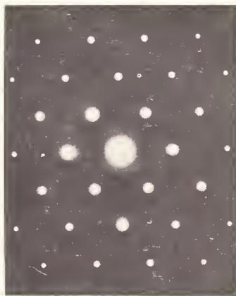
Fig. 3. Transmission electron diffraction pattern obtained from (110) foil of a single crystal TaC_{0.83} sample which had been given a heat treatment similar to that used to develop the ordering in NbC_{0.84} . The presence of diffuse bands, rather than discrete superlattice spots, suggests that the ordering is very imperfect.
