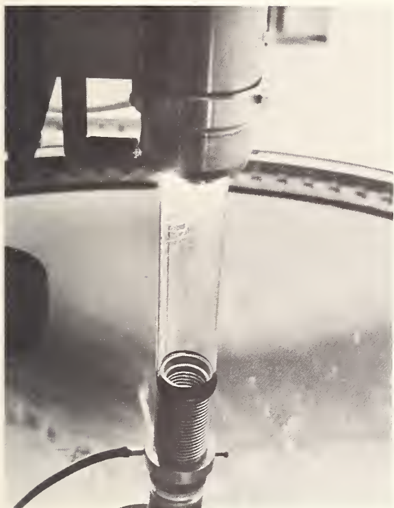
Fig. 3. View of the spitting phenomena occurring at the solidification of CoO after melting in pure oxygen.
