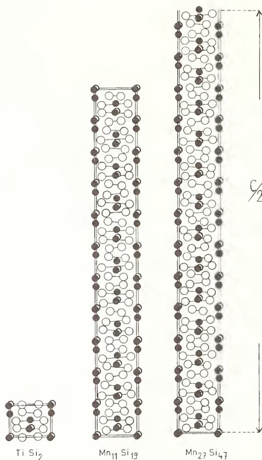
Fig. 10. Atomic arrangement of \text{TiSi}_2 , \text{Mn}_{11}\text{Si}_{19} and \text{Mn}_{27}\text{Si}_{47} .
