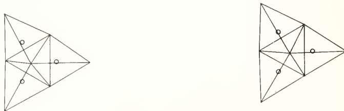
Fig. 7. Stereoscopic view of 3 FeSe_4 tetrahedra forming the trinuclear unit in Ba_3Fe_3Se_7 .
