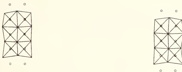
Fig. 3. Stereoscopic drawing of the double tetrahedral chain in \text{BaFe}_2\text{S}_3 . The horizontal direction is [100] and the vertical [001] .
