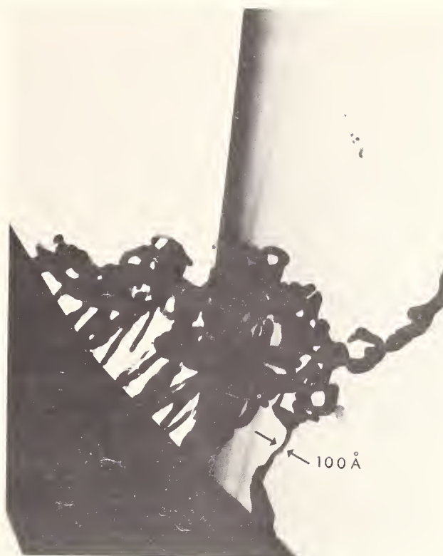
Fig. 11. Enlargement showing detail in whiskers growing from silver beta alumina.
