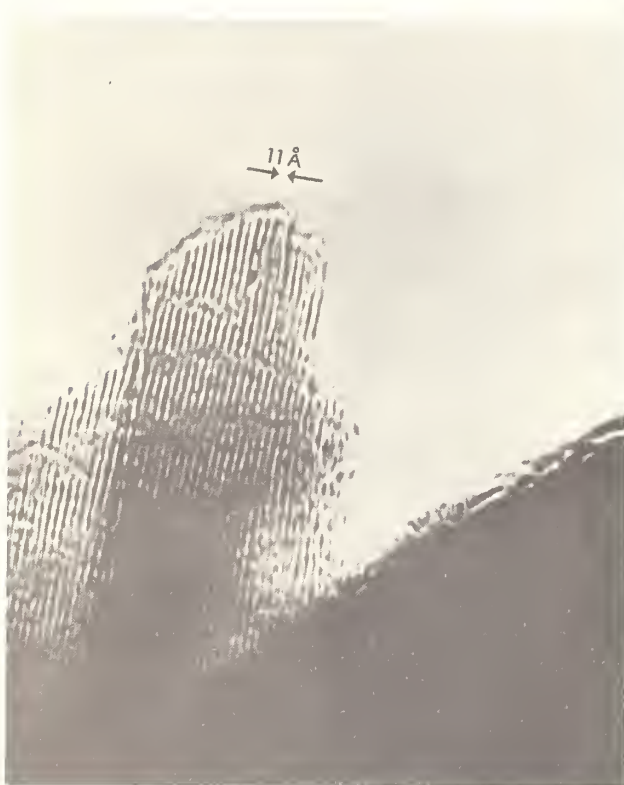
Fig. 4. Lattice fringes corresponding to (00.2) planes in beta alumina. The fringe separation is about 11 Å.
