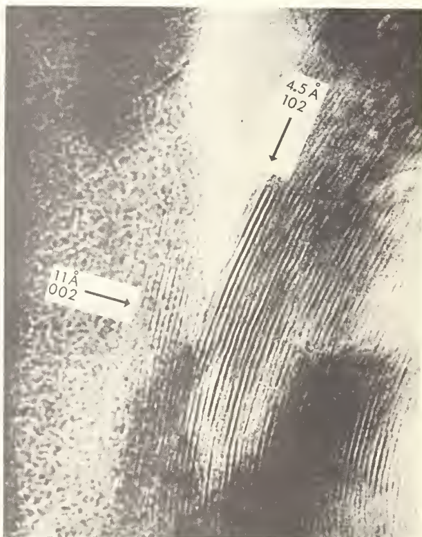
Fig. 5. Beta alumina cross grating pattern. Wide fringes are (00.2) planes ( d=11.3 Å) and fine fringes are (10.2) planes ( d=4.45 Å). Note curvature of the (00.2) planes.
