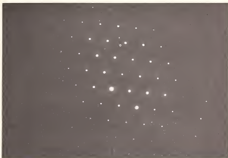
Fig. 4. Electron diffraction of a crystal of A-Nd 2 O 3 . The electron beam is along the c -hexagonal axis. Plane of the thin film is parallel to (00.2).
