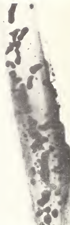
Fig. 8. Electron micrograph of silver beta alumina crystal corresponding to diffraction pattern in figure 7.
