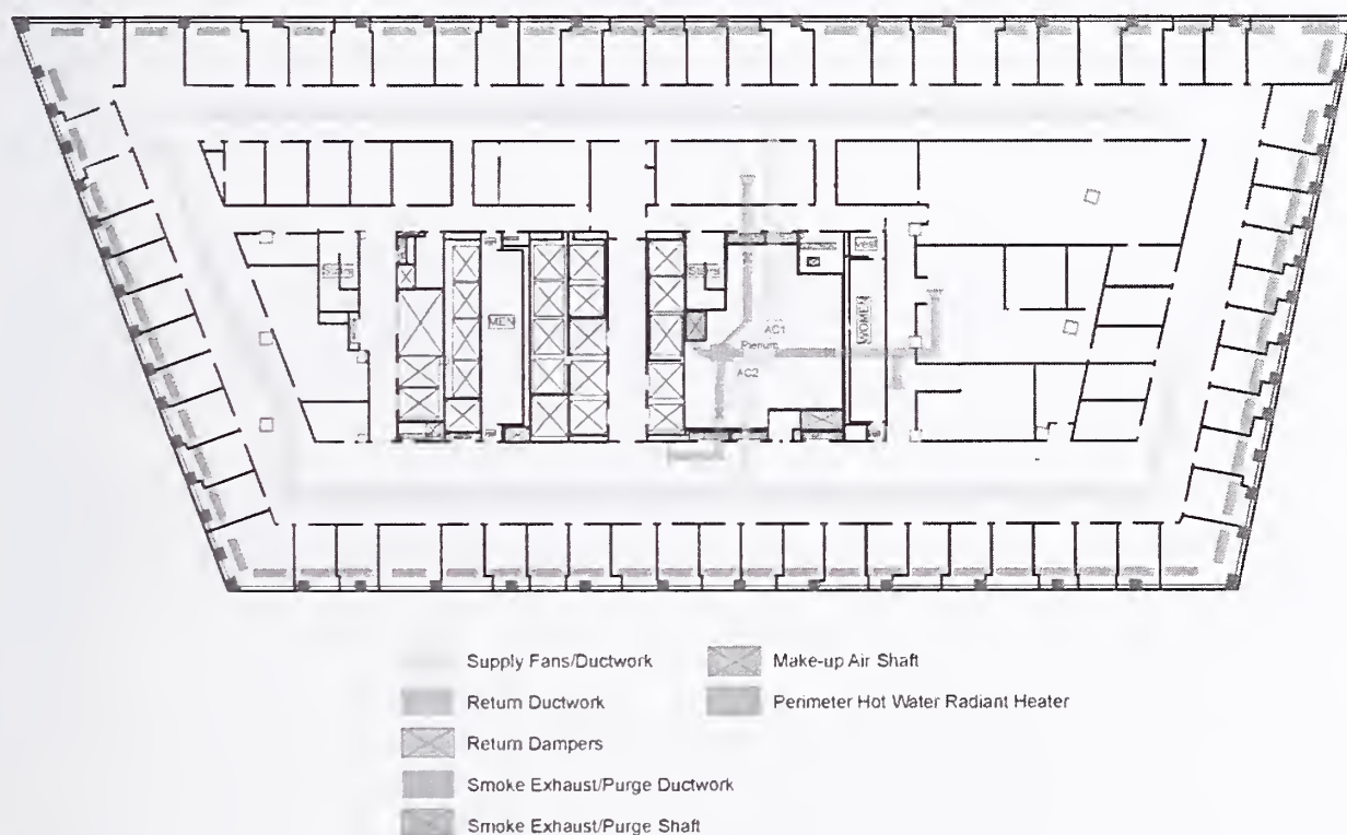
Figure 4-11. Air distribution system, 24th floor, WTC 7.
