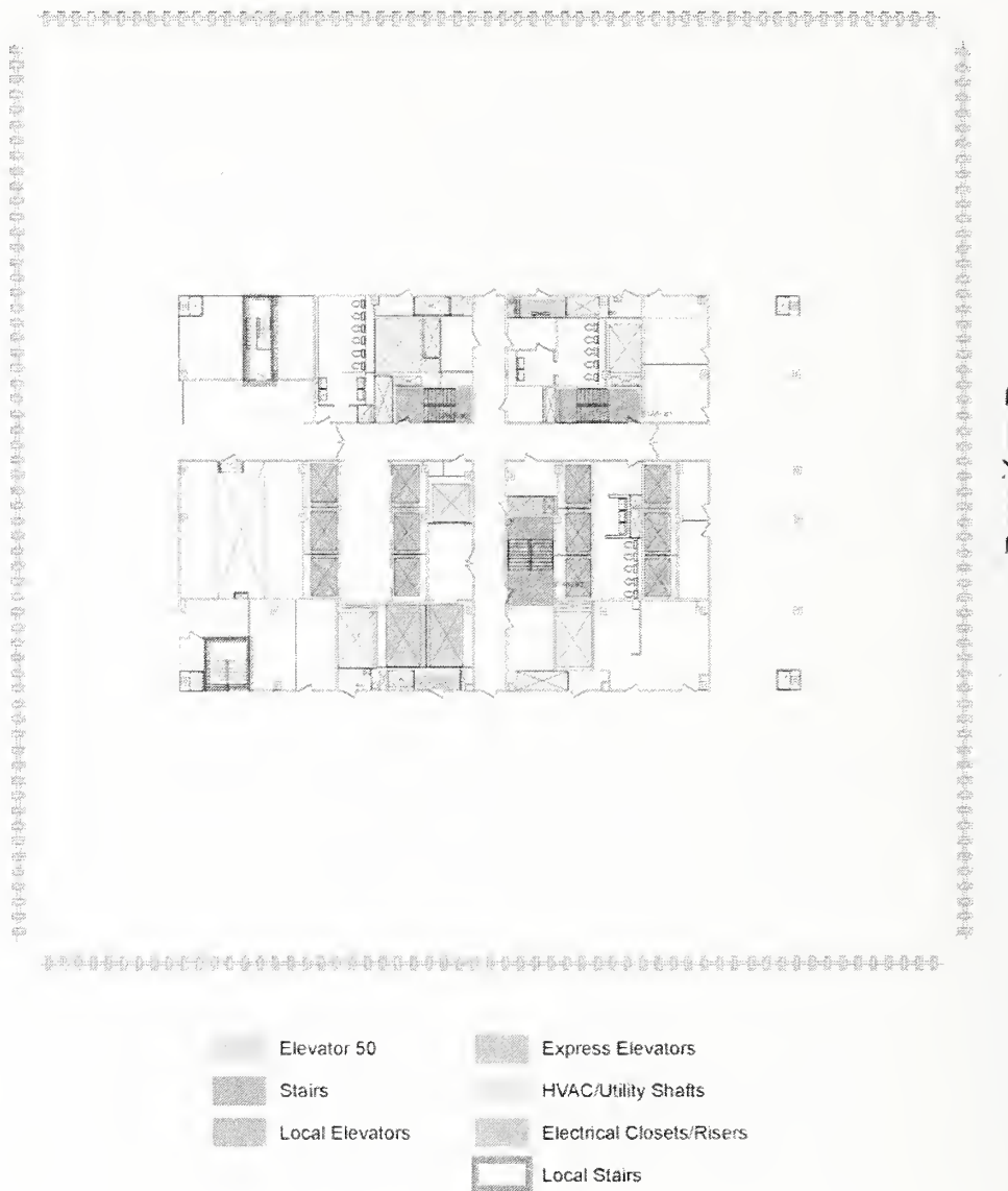
Figure 4–1. Floor layout, 95th floor, WTC 1.
