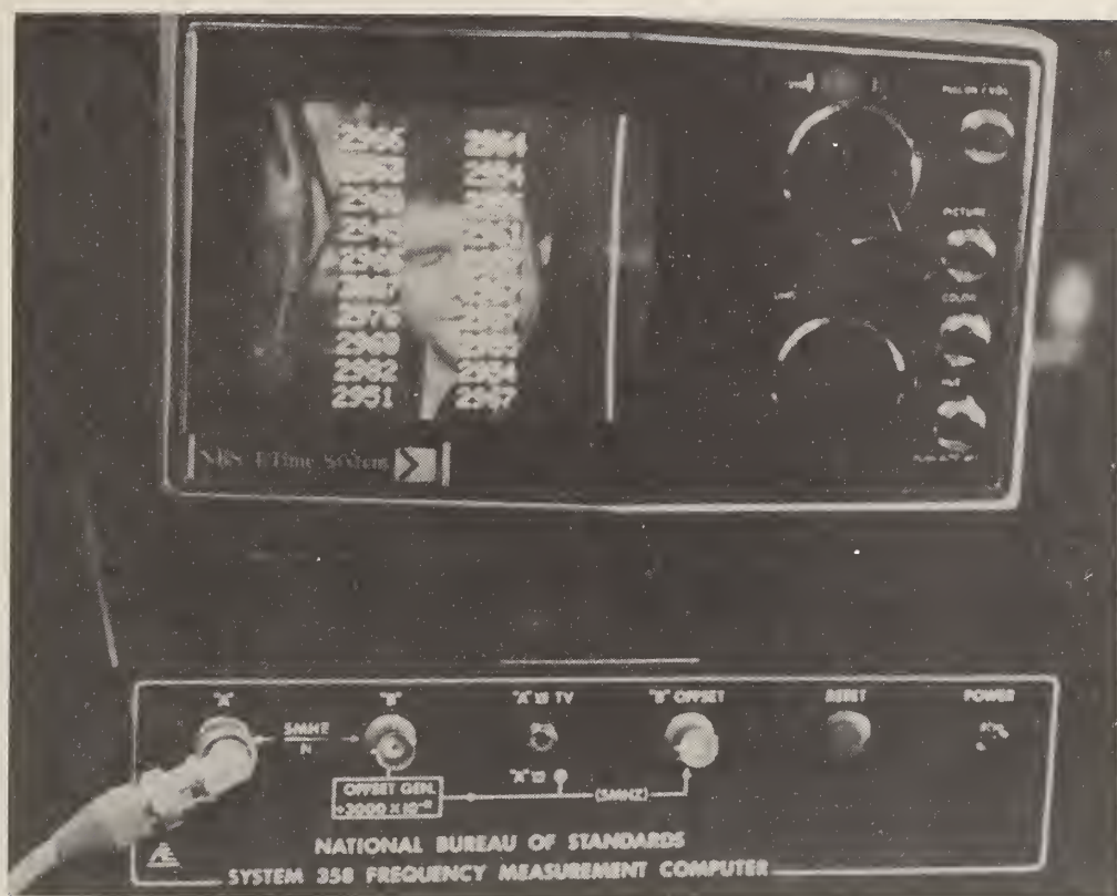
FIGURE 7.5. THE NBS PROTOTYPE, SYSTEM 358 FREQUENCY MEASUREMENT COMPUTER.
