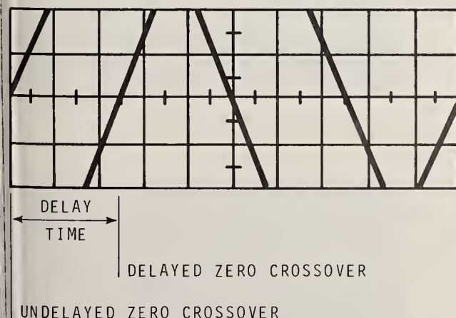
FIGURE 5.14. OSCILLOGRAM OF DELAYED AND UNDELAYED 1 kHz SIGNAL.
