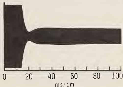
FIGURE 6.17. WWVB ENVELOPES AS TRANSMITTED.
