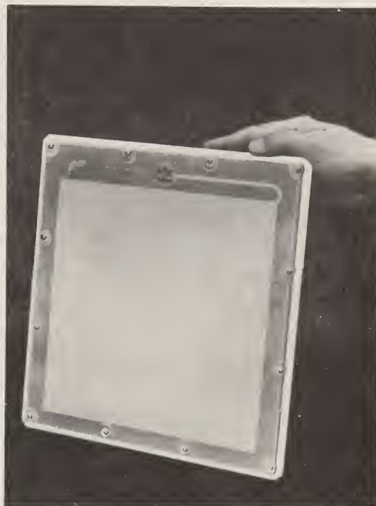
FIGURE 10.10. MICROSTRIP ANTENNA USED TO RECEIVE GOES TIME CODE.
