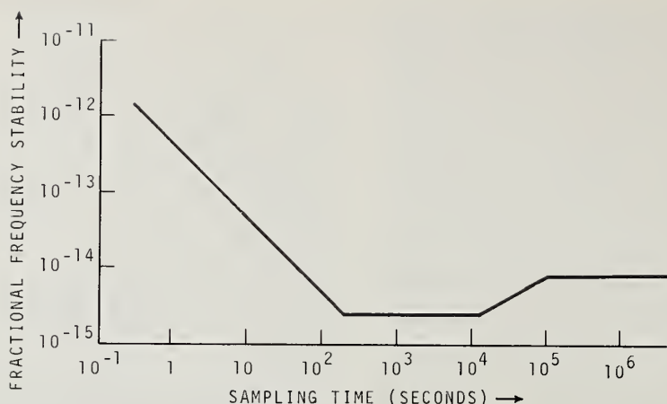
FIGURE 11.26. FREQUENCY STABILITY OF A HYDROGEN MASER OSCILLATOR.
