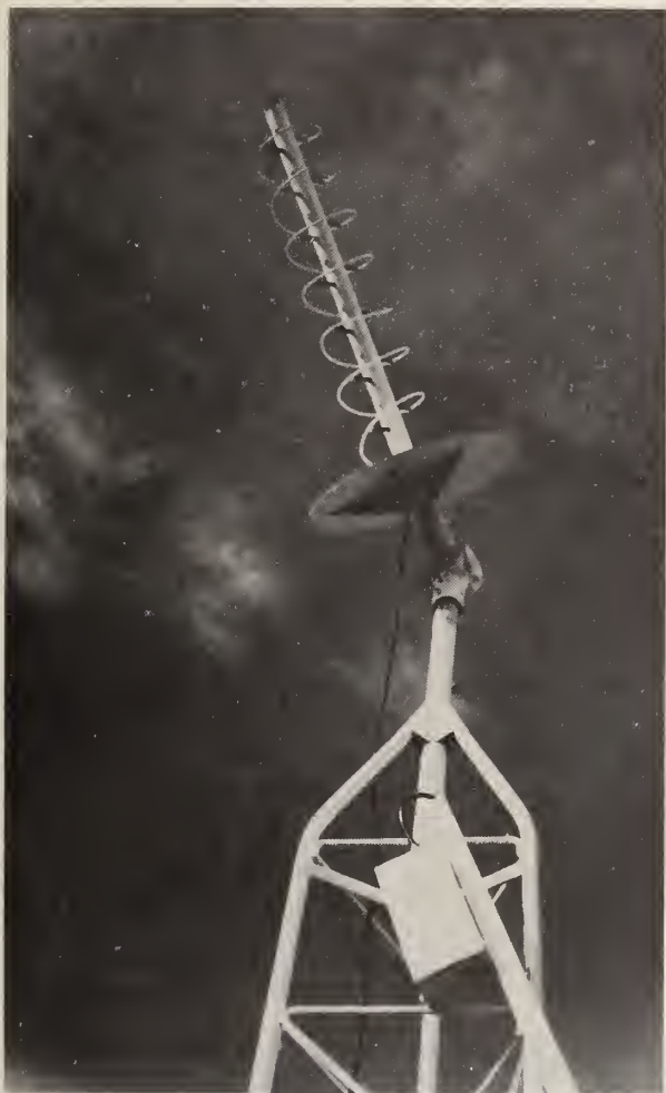
FIGURE 10.9. RIGHT-HAND CIRCULARLY POLARIZED HELIX ANTENNA USED TO RECEIVE GOES SIGNALS.
