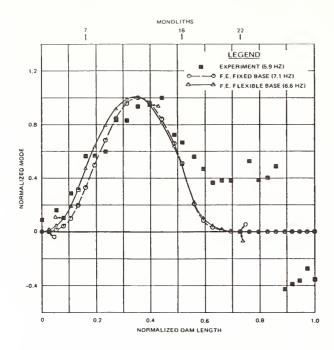
Figure 7. Mode 1 - Dam without Reservoir.
