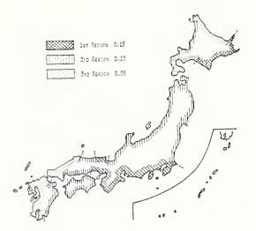
Fig.6 Seismic Zoning Map for Port Structures
