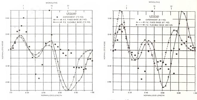
Figure 15. Mode 4 - Dam with Reservoir.
