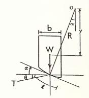
Fig.4 Slice for a Circular Slip Surface Analysis
