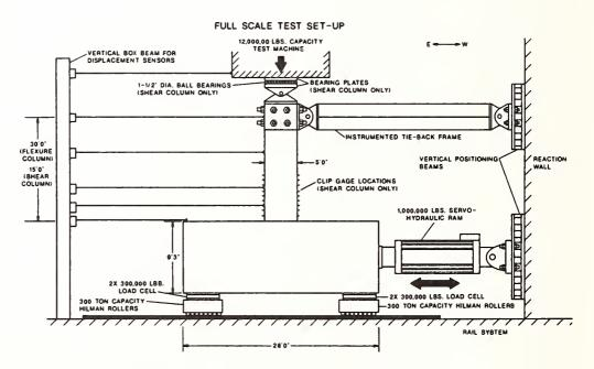
Figure 4: Schematic of Full-Scale Test Apparatus
