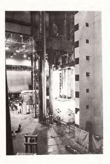
Figure 5: Prototype Shear Column Under Test in NBS Large Scale Structures Laboratory.
