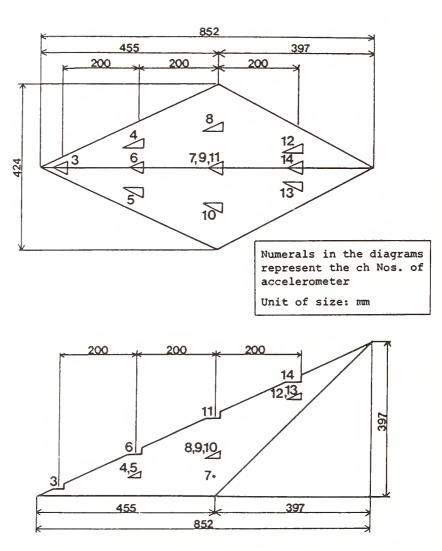
Fig. 2 Locations of Accelerometers (Case 1)
