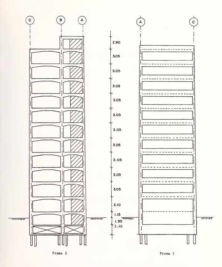
Figure 3 Elevation views of Frame 2 and Frame 1 before retrofit
