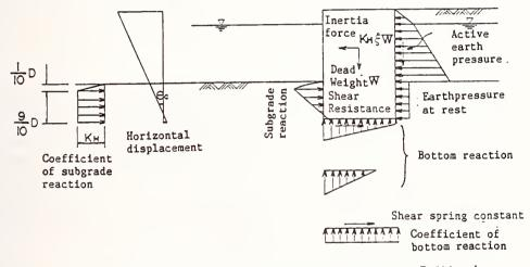
Fig.15 Calculation Model of Steel Plate Cellular Bulkhead
