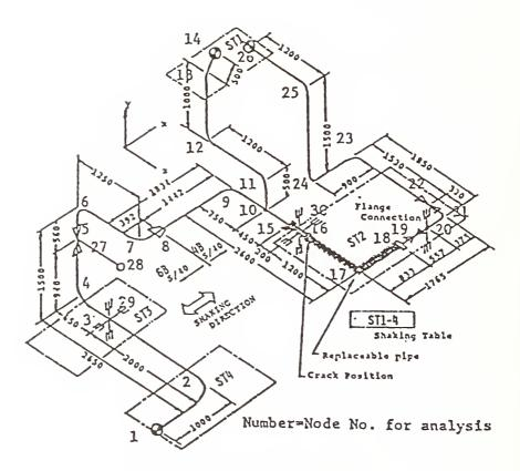
Fig. 17. Test Piping Model
