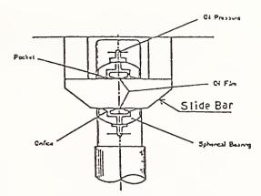
Fig. 19. Hydraulic Actuator with Joint
