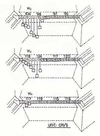
Fig. 15 Sliding of Submerged Caissons
