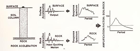
Figure 1.--Schematic illustration showing (from left to right) the soil-rock column, the bedrock and surface acceleration time histories, the corresponding response spectra derived from them, and the spectral amplification factor transfer function). The peak amplitude of acceleration is read from the acceleration time histories. The soil-to-rock amplification factor for a discrete period band is read from the transfer function.
