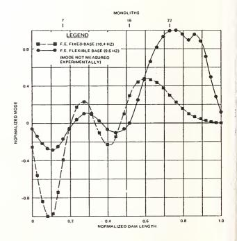
Figure 10. Mode 4 - Dam without Reservoir.
