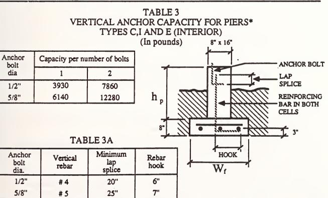
\* The vertical anchor capacity is based upon the working capacity of ASTM A - 307 anchor bolts in 2500 psi concrete or grout. To fully develop this capacity, anchor bolts must be properly connected to the foundation and superstructure. <sup>1</sup>The capacity is based on  $F_c = 2500$  psi;  $f_v = 40,000$  psi
