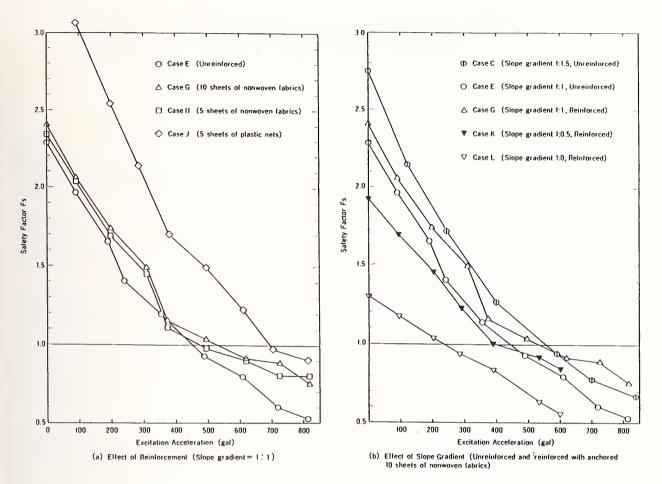
Fig.6 Relationship between Excitation Acceleration and Safety Factor
