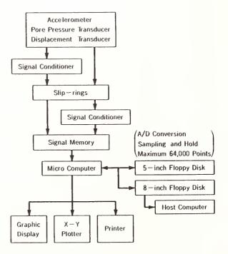
Fig.6 Schematic of Data Measurement System
