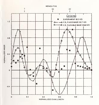
Figure 11. Mode 5 - Dam without Reservoir.
