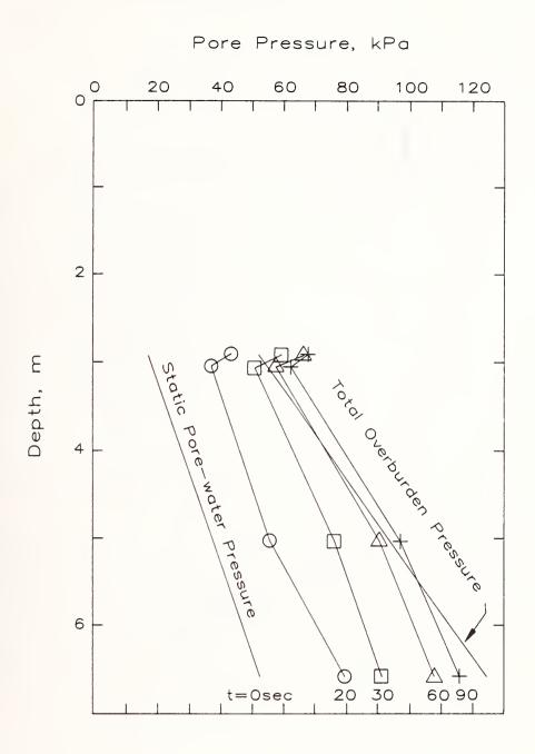
Figure 6. Pore pressure versus depth for selected times after the earthquake triggered the Wildlife array. Zero time is when the recorder triggered.
