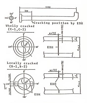
Fig. 18. Drawing of Pipe Cracks
