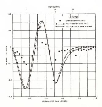
Figure 9. Mode 3 - Dam without Reservoir.
