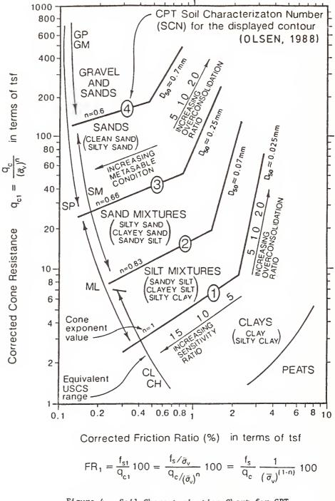
Figure 4. Soil Characterization Chart for CPT (from Olsen, 1988)
