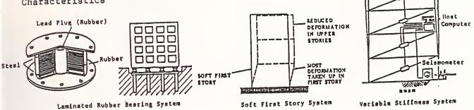
ii) A Method to Control and Adjust Damping
