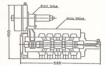
Fig. 22. Section of Servo Valve
