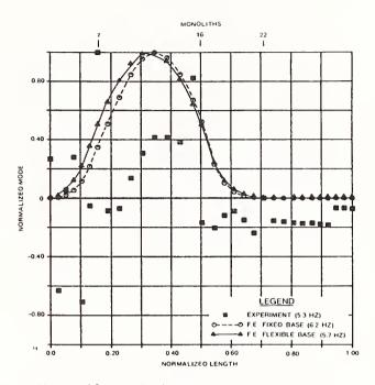
Figure 12. Mode 1 - Dam with Reservoir.
