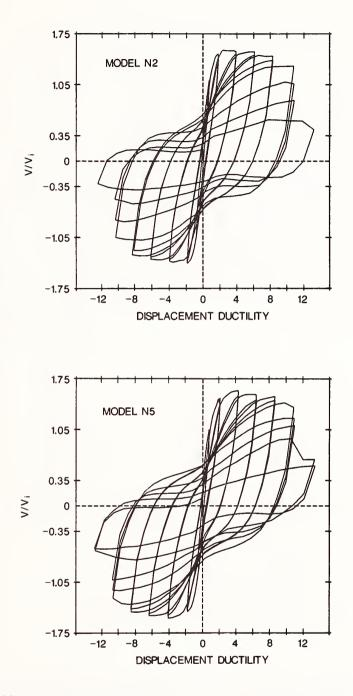
Figure 10c: Normalized Lateral Load  $(V/V_i)$  versus Displacement Ductility  $(\Delta/\Delta_y)$  for 1/6-Scale Model Shear Columns. N2 = microconcrete; N5 = readymix;  $P_e/(f'_cA_g) \approx 0.2$
