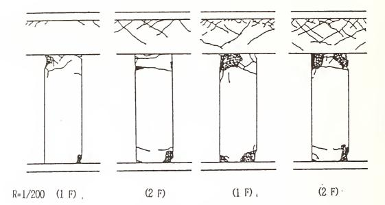
Fig. 9 Crack Pattern of Infilled Wall ( B Frame)
