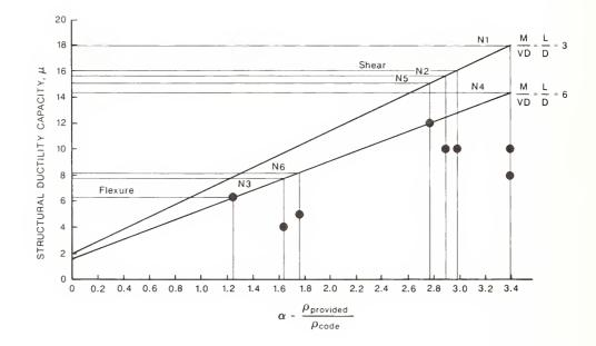
Figure 11: Structure Ductility Capacity Related to Confinement Ratio
