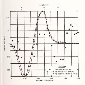
Figure 13. Mode 2 - Dam with Reservoir.
