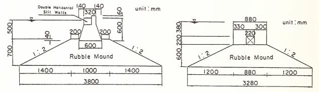
Fig. 5 Cross Sections of Breakwaters
