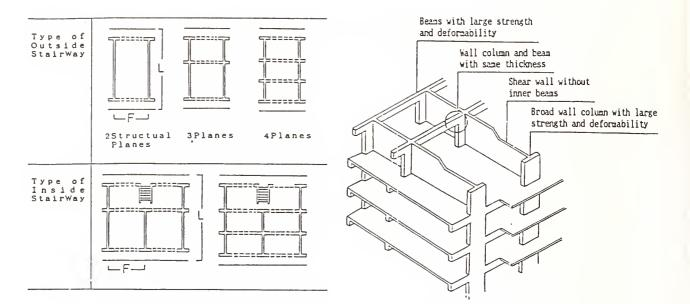
Fig. 2.1 Example of Typical Plan
