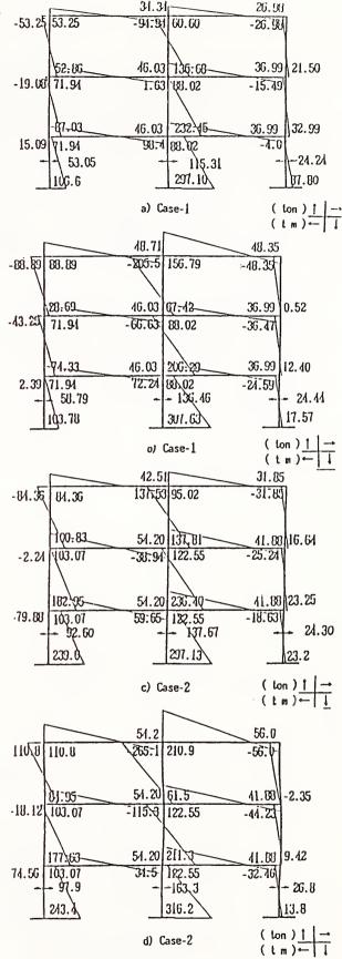
Fig. 14 Noment Diagram at Hinge Nechnism
