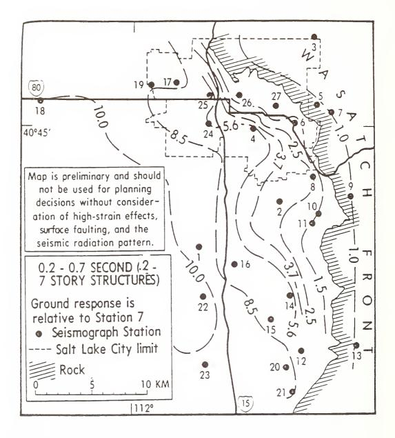
Figure 10.--Map showing the site amplification factor for the period band 0.2-0.7s, Salt Lake City area. Values on contours indicate the radios of velocity response spectra that would be expected relative to rock on the Wasatch Front. These values provide an estimate of the spatial variation of ground motion in the period band in which the 2-7 story buildings have their fundamental natural period of vibration.
