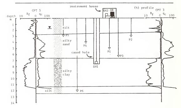
Figure 3. Cross section and map view of liquefaction array (Bennett and others, 1984). Units of  $R_f$  and  $q_c$  are per cent and kg/cm<sup>2</sup>, respectively.
