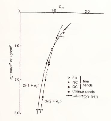
Figure 3. Overburden correction curves for fine and coarse sands (from Skempton, 1986)
