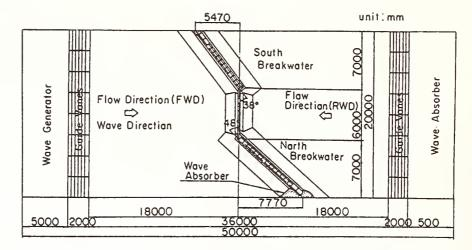
Fig. 4 Breakwater Arrangement in Experimental Basin
