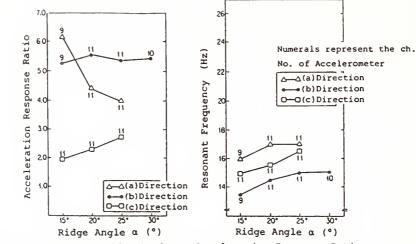
Fig. 9 Effect of Ridge Angle on Acceleration Response Ratio and Resonant Frequency
