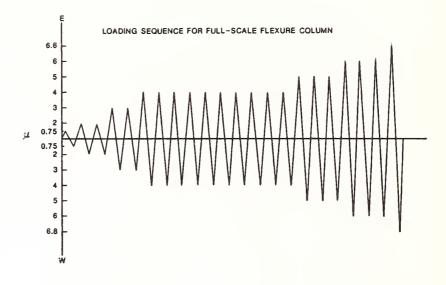
Figure 6a: Loading History for Flexure Columns
