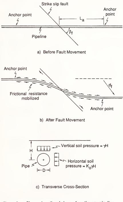
Figure 2. Plan and sectional views of continuous pipeline envisioned in Newmark-Hall design approach.
