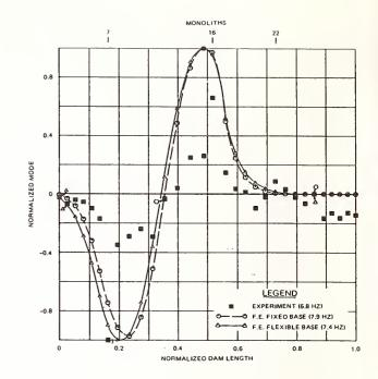
Figure 8. Mode 2 - Dam without Reservoir.
