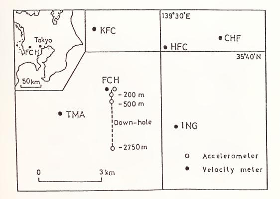
Fig. 13. Layout of Seismographs at the Fuchu Area
