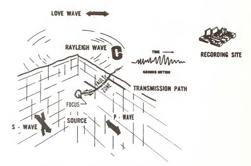
Figure 3.--Schematic illustration showing the earthquake-path-site-structure system.
