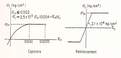
Fig. 3 Stress-Strain Diagram of Concrete and Reinforcement
