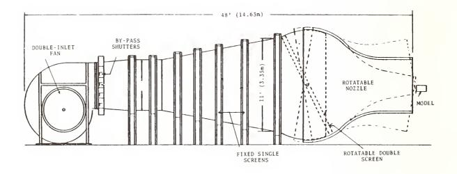
FIGURE 4. LINE DRAWING OF WIND TUNNEL
