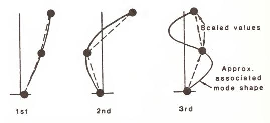
Figure 3. Sketch of the lower translational modes sought for moderately instrumented buildings.
