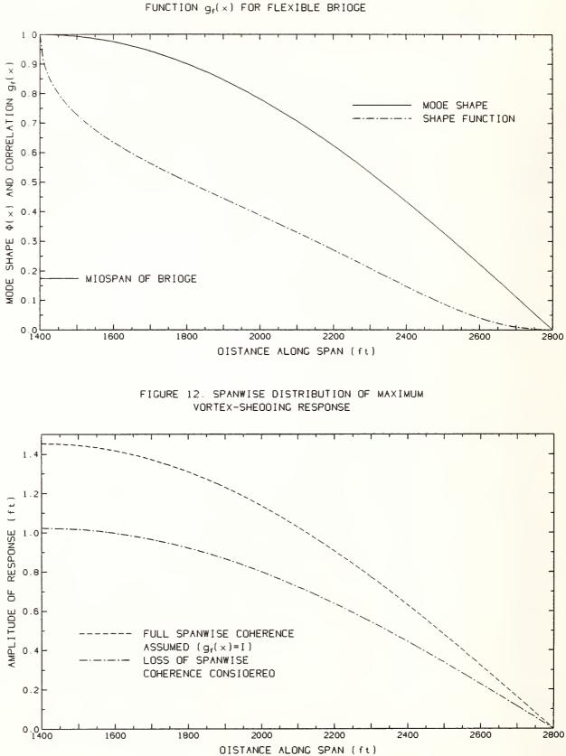
FIGURE 11. MODE SHAPE  $\Phi(\,\times\,)$  AND CORRELATION (SHAPE)
