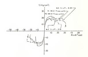
Fig.4.6 τ versus R relations (Effect of transverse wall and axial stress level)
