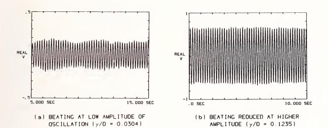
FIGURE 13. SAMPLES OF VERTICAL RESPONSE AT LOCK-IN
