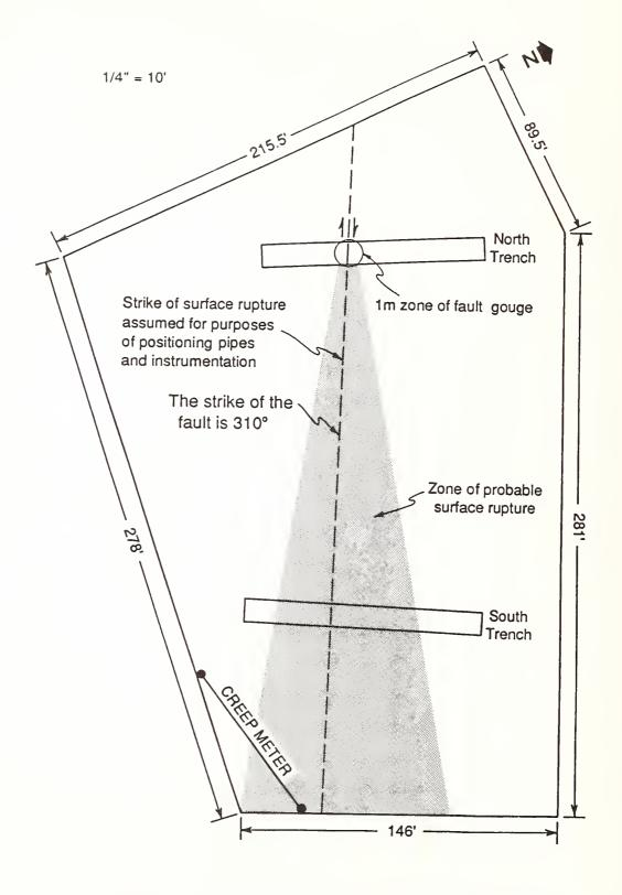
Figure 3. Assumed zone of surface rupture, Owens Pasture.
