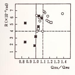
Fig. 3.7 Shear Strength-Ratio v.s. Deformation Capacity
