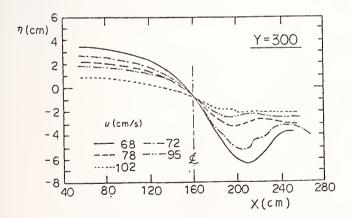
Fig.9 Water Surface Profiles at Y=300
