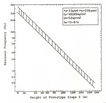
Fig. 11 Resonant Frequency Estimation of Prototype Slope
