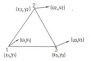
Fig. 3 Element for Strain Calculation
