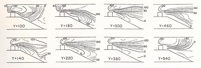
Fig.7 Equi-velocity Contours in Vertical Sections
