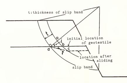
Fig.5 Calculation of Tension of Geotextile
