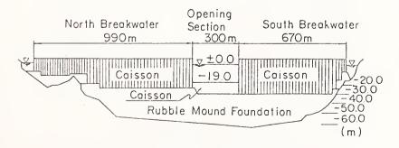
fig.3 Longitudinal Section of Breakwaters
