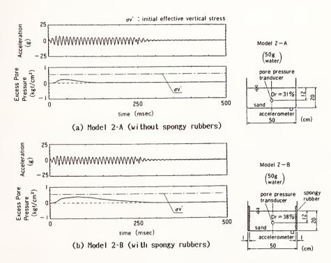
Fig.8 Effect of the Restraint of End Walls
