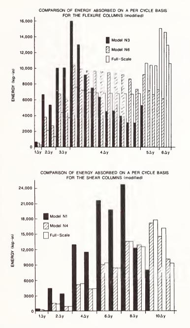
Figure 12: A Comparison of Cyclic Energy Dissipation between Model and Prototype Specimens with Modifications to Account for Differences in Compressive Strength between Models and Prototypes, and for Friction Losses in the Prototype Tests. Top Chart is for Flexure Specimens (L/D = 6); Bottom Chart for Shear Specimens (L/D = 3).
