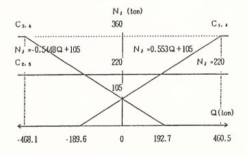
N<sub>s</sub> : appling axial force/one column
