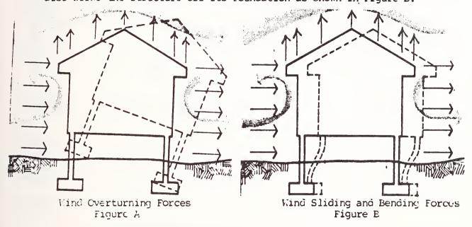
High wind forces tend to stress the connections between structural members, such as those connecting floor beam girders and those connecting them to vertical supports. Such stresses may cause a progressive weakening of these connections to the point where failure is possible.
