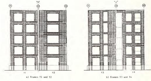
Fig.5 Reinforcement Layout in Lateral Resisting Frames
