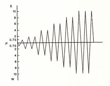
Figure 6b: Loading History for Shear Columns
