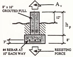
\* Potential withdrawal resistance is the maximum uplift resistance which can be provided by the foundations shown. It is computed by adding the weights of building materials and soil over the top of the footing. To fully develop this potential, adequate connections to the footing and superstructure must be provided.
