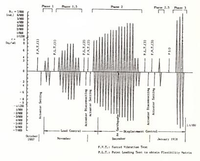
Fig.12 Loading Sequence through Overall Testing
