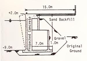
Tig.5 Cross Section of Cellular block Quaywall (Akita Port)
