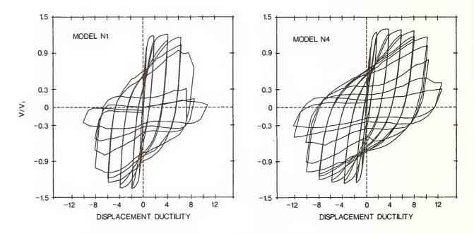
Figure 10b: Normalized Lateral Load (V/V<sub>i</sub>) versus Displacement Ductility  $(\Delta/\Delta_y)$  for 1/6-Scale Model Shear Columns. N1 = microconcrete; N4 = readymix; P<sub>e</sub>/(f'<sub>c</sub>A<sub>g</sub>)  $\approx$  0.1
