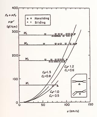
Fig. 16 Stability of Submerged Caisson
