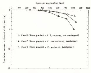
(b) Effect of Anchorage and Overlapping (10 sheets of nonwoven fabrics)
