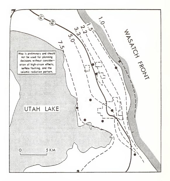
Figure 12.--Map showing the site amplification factors for the period band 0.2-0.7s, Provo area. Values on contours indicate the ratios of velocity response spectra that would be expected relative to rock on the Wasatch Front. These values provide an estimate of the spatial variation of ground motion in the period band in which the 1-7 story buildings have their fundamental natural period of vibration.
