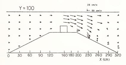
Fig. 8 Velocity Vector at Section of Y=100
