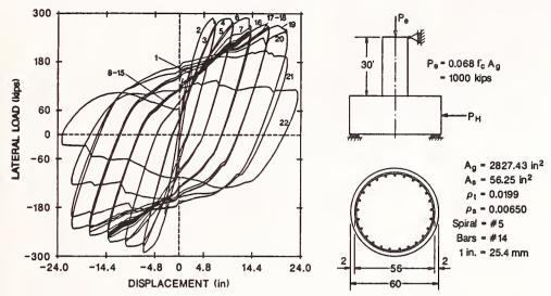
Figure 7a: Lateral Load vs. Displacement plot for Full-Scale Flexure Column. Cycle Numbers 1,2,4,6,16, and 19 correspond to Displacement Ductilities of 1,2,3,4,5, and 6, respectively
