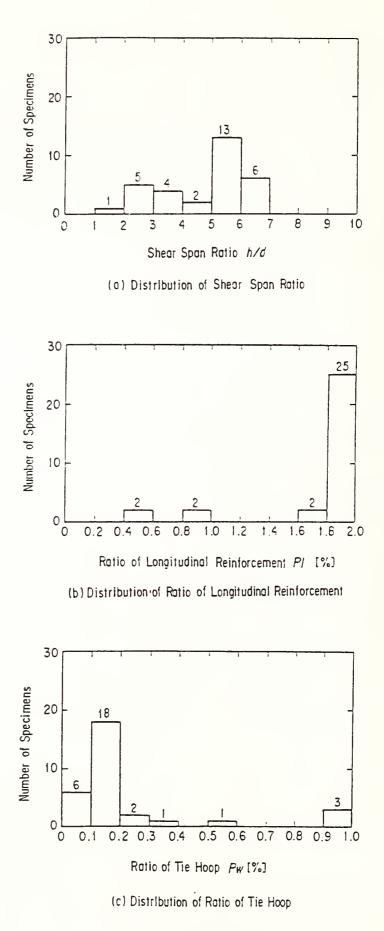
Fig. 1 Feature of Specimens
