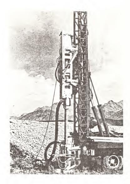
Figure 1. Photograph of Becker Hammer Drill Rig (From Harder and Seed, 1986)
