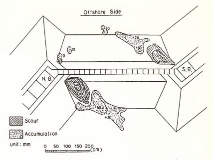
Fig.10 Deformation of Rubble Mound Foundation
