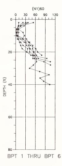
Figure 9. Becker Hammer soundings in undisturbed alluvium of the American River valley
