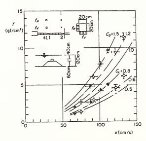
Fig.13 Hydrodynamic Forces vs Velocity
