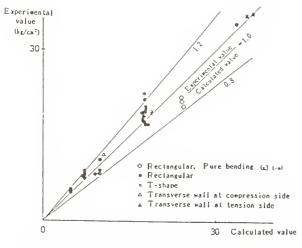
Fig.4.1 Maximum flexural strength  $(\tau_{HU}=M_{U}/(bDh))$
