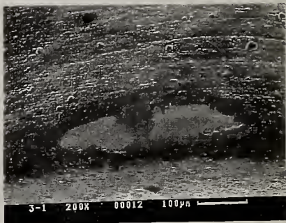
Fig. 11. SEM of a Worn Through Insert
