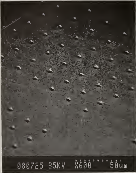
Fig. 1 Array of diamond pyramids on diamond.
