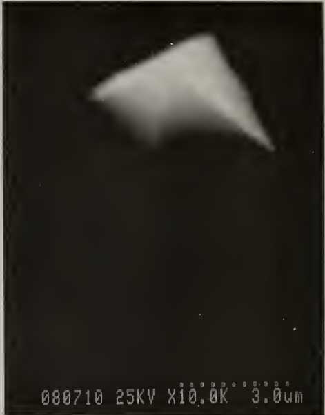
Fig. 2 A single pyramidal microtip on diamond.
