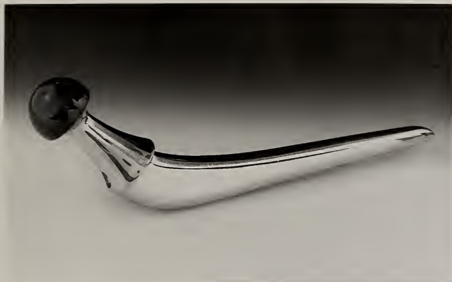
Fig 1. DLC coating of the femoral head of a hip prosthesis
