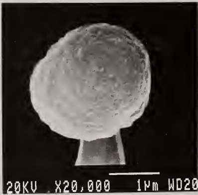
Fig. 2. Various microstructures of particles on tip ends: a - fine-crystalline; b - large-crystalline particles.
