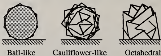
Figure 2 Evolution of morphological structures in diamond deposition
