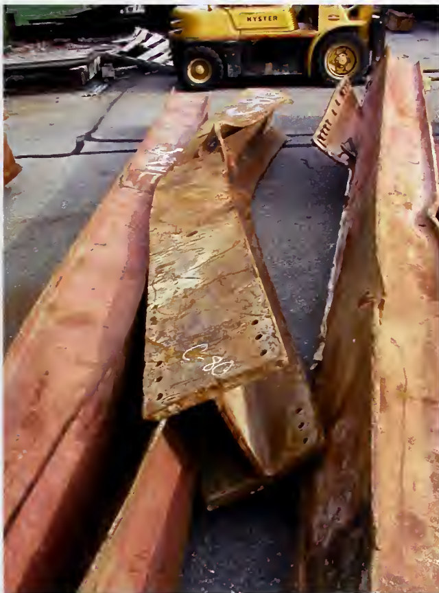
Figure 1-8. Recovered wide flange sections used as core columns.
