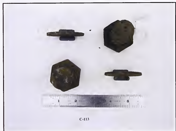
Figure 1-13. Examples of recovered bolts from various samples.
