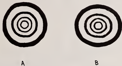
Figure 6. Synthetic interferograms for isotropic (A) and anisotropic (B) effects. \chi_A = 0 for (A) and \chi_A = 0.2 for (B). \chi_I = 1 for both cases.
