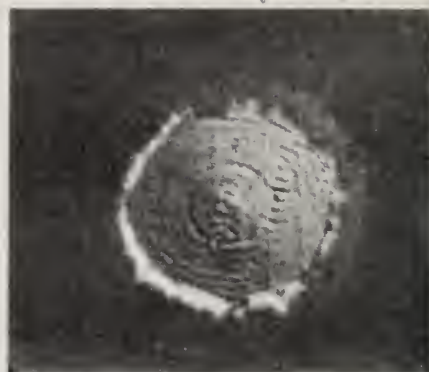
Figure 9. Effects of surface defects on window coating damage (exit surface). Note that the ripple pattern is associated with the coating separation line. The laser spot 1/e^2 diameter was 200 μm. As in all the micrographs presented here, the incident laser electric field is in the vertical direction.
