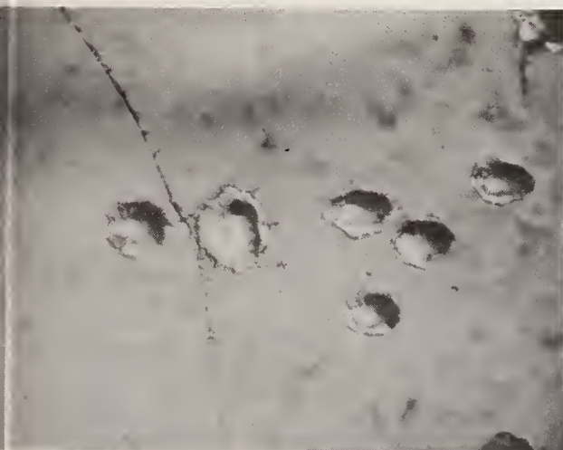
Figure 6. Nomarski micrograph of damage to entrance surface of h-p \text{CdCr}_2\text{S}_4 caused by hot spots in shot 2; 750x - micrograph spans 150 \mu\text{m} of surface.
