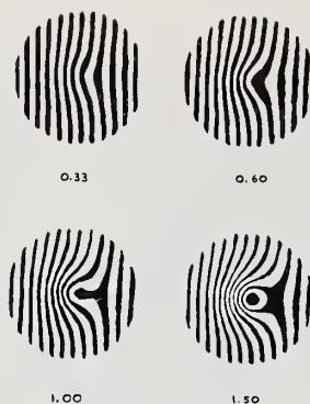
Figure 8. Synthetic interferograms showing effect of changing X_I . The reference fringe bias was a simple wedge (straight line fringes).
