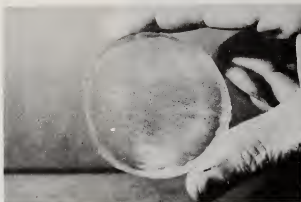
Figure 5. Photograph showing veils in a \text{CaF}_2 crystal forged at 650^\circ\text{C} .
