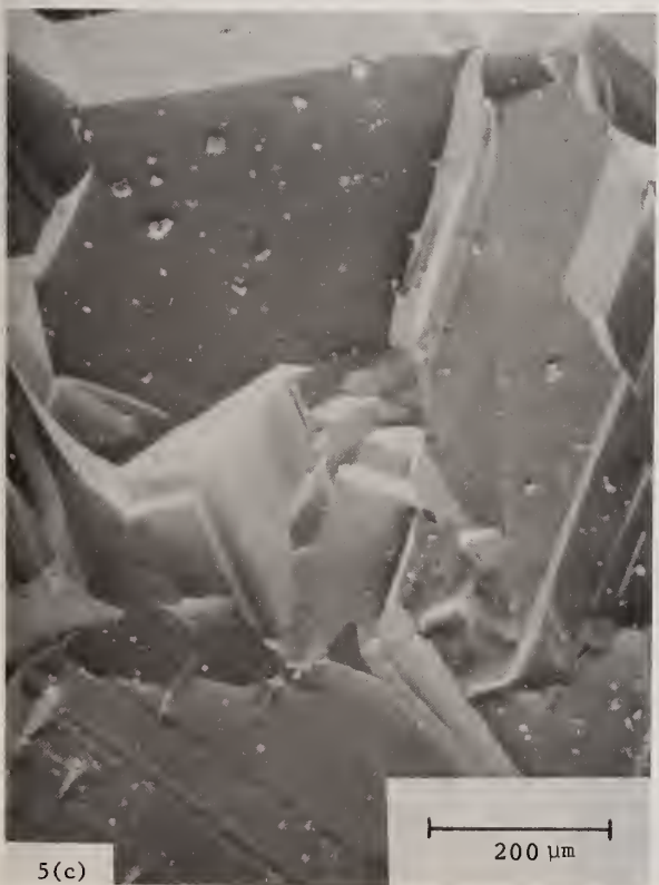
Figure 5. SEM micrographs of as-deposited surfaces, (a) sample KU-8-3 (grown under conditions of high Q ) shows high degree of faceting and voids at grain boundaries; (b) sample KU-7-3, and (c) sample KU-13-5 (grown with protective silica tube) both grown under conditions of low Q exhibit lower degree of faceting with no apparent voids at boundaries.
