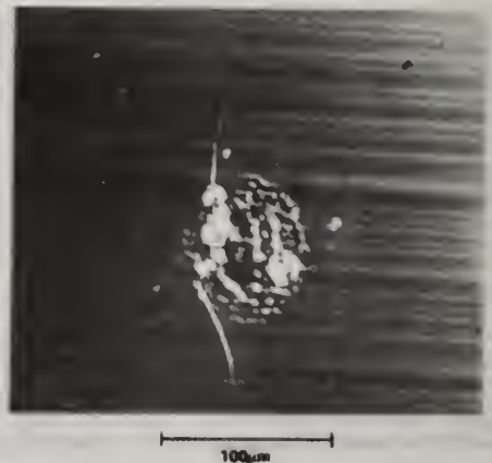
Figure 8. Nomarski micrograph of another damage site on LLL Cu 8B, considerably above threshold for that site.
