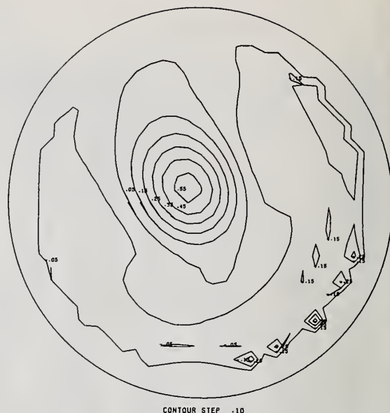
Figure 9. OPD contours for optical distortion in barium fluoride. Contour step is fractions of He-Ne laser wavelength ( .6328 \mu\text{m} ).
