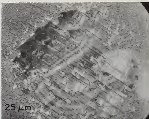
Figure 4. Nomarski micrographs of entrance surface damage to \text{CaF}_2 . The lower photograph is an enlargement of the damage site showing the aligned cracks.
