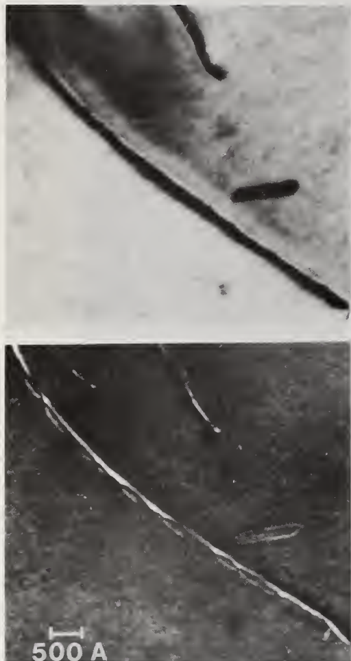
Figure 19. (a) Bright-field view of dislocation in sample 2. (b) Corresponding weak-beam dark-field image showing dislocation dissociation. Diffracting condition is chosen so that both partials are in contrast.
