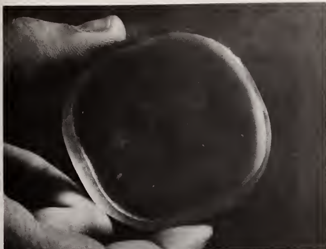
Figure 2. KCl forging \langle 100 \rangle orientation deformed 60% without Teflon (left side).
