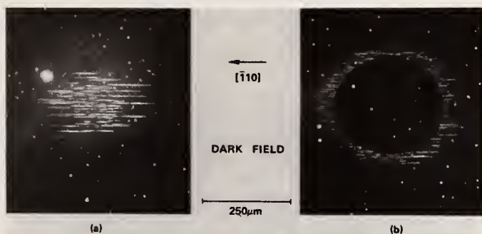
Figure 8. Damage on the Al(110) target below (a) and above (b) the threshold for crater formation, as seen in dark field micrographs. Exposure is 12.2 \text{ J/cm}^2 (max. of 2 pulses) in (a) and 16.9 \text{ J/cm}^2 (one pulse) in (b).
