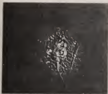
Figure 9. Nomarski micrograph of a damage site on LLL Cu 8B, after being mechanically polished at NWC following an initial series of damage tests on the diamond-turned surface.
