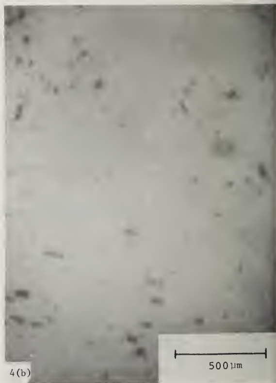
Figure 4. IR photomicrographs of (a) sample KU-6-3 (grown under near stoichiometric conditions) showing significant concentrations of large voids and (b) sample KU-2-2 grown under Cd rich conditions) showing greatly reduced size and concentration of voids.
