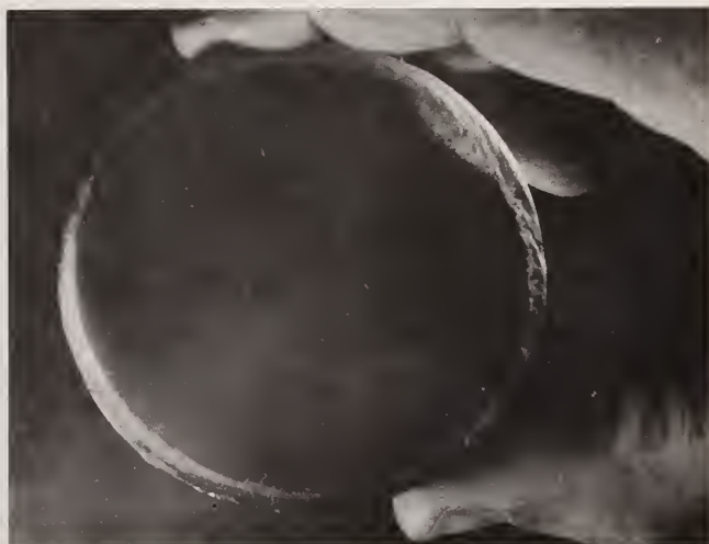
Figure 2. KCl forging \langle 100 \rangle orientation deformed 60% with Teflon (right side).
