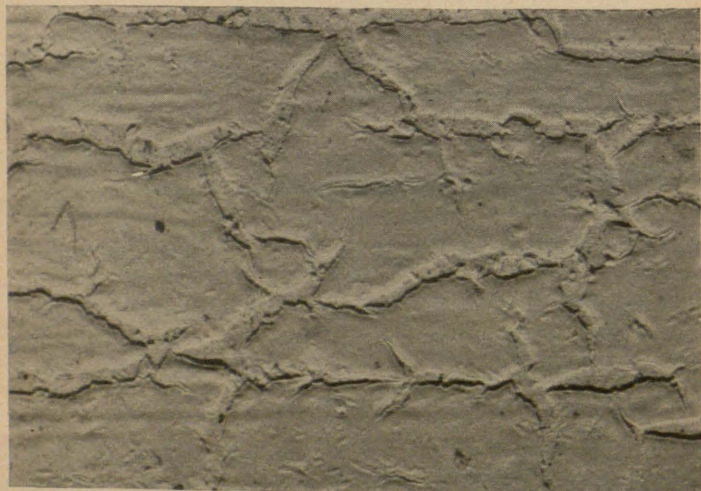
FIGURE 24.— Additional example of alligatoring of paint.
