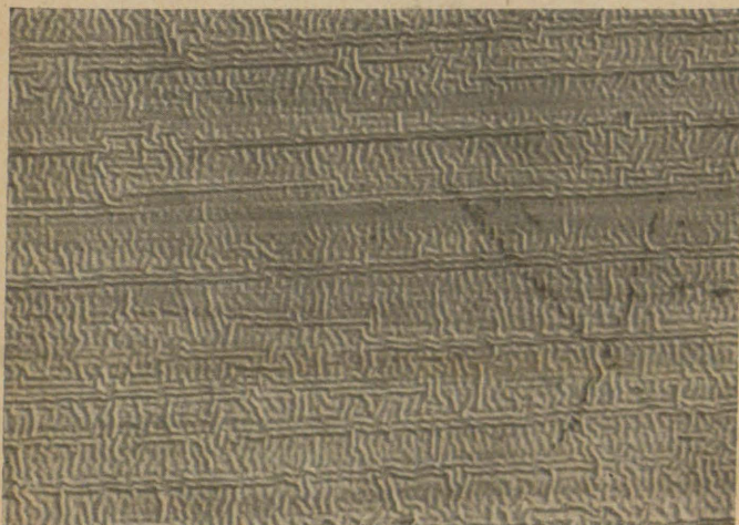
FIGURE 22.— Paint that has wrinkled soon after application.
