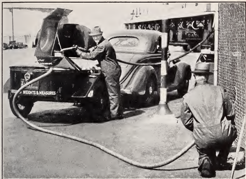
FIGURE 1.—50-gallon standard measure.
