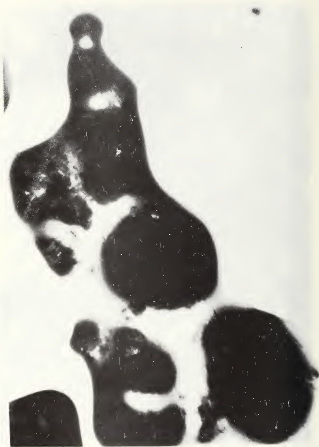
Figure 11. Soluble salts extracted from Tumacacori specimen To 11 . This salt sample was dried at 105°C to constant weight and then exposed to laboratory air (23°C, 35% r.h.) for 30 minutes. 65X magnification. Transmitted polarized light.
