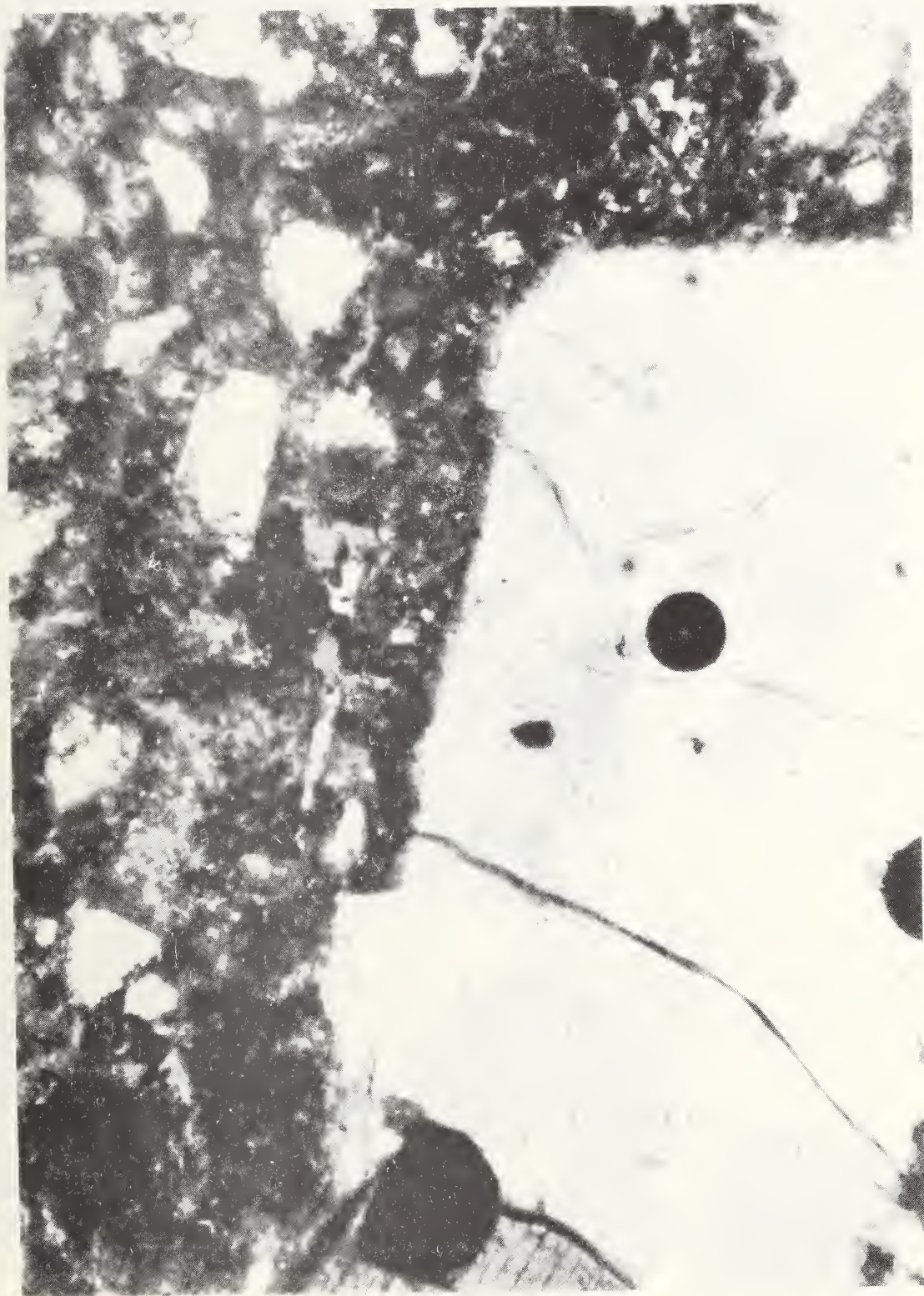
Figure 10. Thin section of adobe from Tumacacori showing a chemically zoned feldspar crystal in the silt-clay matrix. Such zoning is common in the detrital feldspars of this locality. Transmitted polarized light. 100X magnification.
