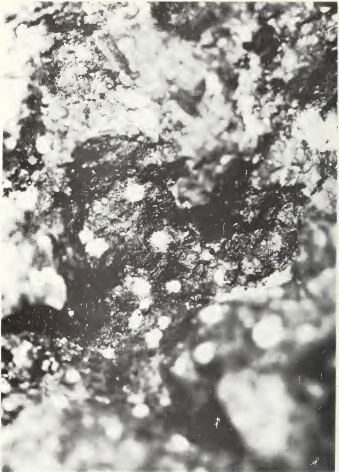
Figure 9. Epoxy-impregnated fracture surface of adobe from Tumacacori showing deposits of gypsum (white) filling the pores. 10X magnification. Sample To 11 .
