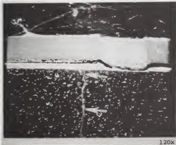
Cross section of base of package showing crack (S.E.M. photo at 120X).
