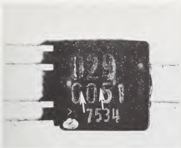
Cracked package (typical) as noted in early 30X visual inspection at vendor's facility.
