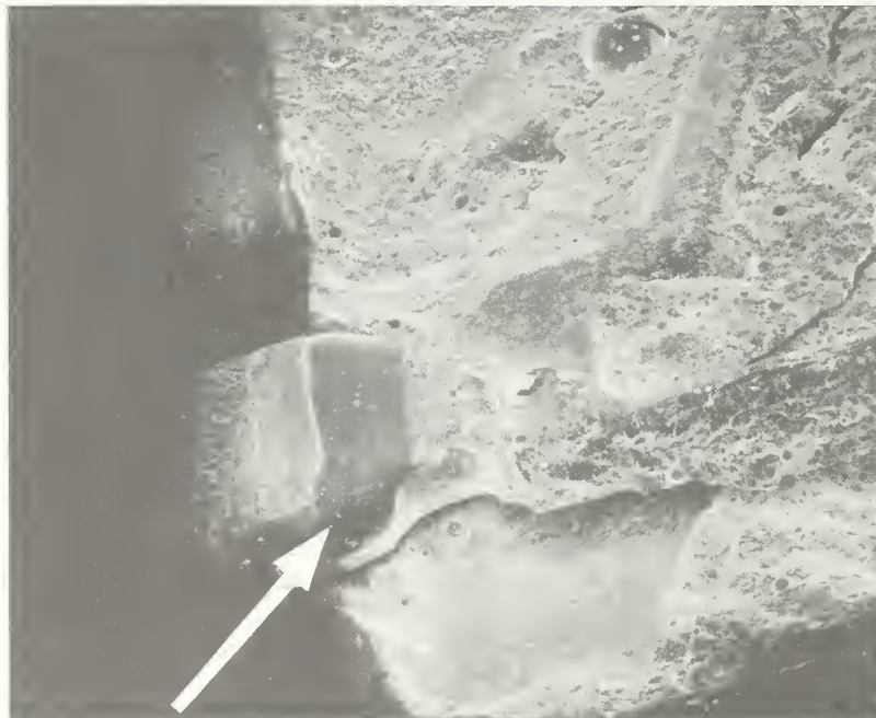
Figure 2. SEM micrograph of single lead frame showing lack of adherence (arrow) of the glass to the bare Kovar while adhering tenaciously to the aluminum-coated portion of the lead frame towards the inside of the package.
