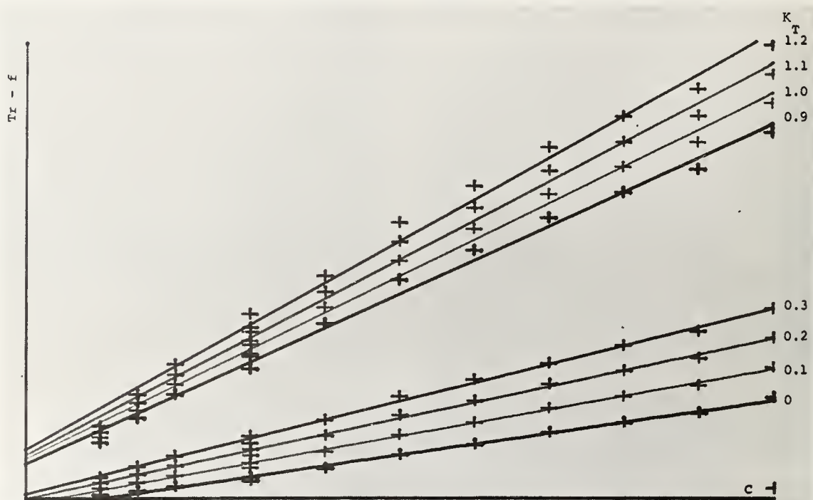
FIGURE 9. Treiber-functions ( Tr-f ) with varying K_T -values at 315 nm for a concentration range 1-10 \mu\text{g}/\text{spot} .
