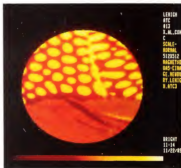
Figure 15. Secondary ion mass spectrometry/ion microscope image of aluminum in an aluminum-lithium-copper alloy. Image diameter = 150 \mu\text{m} .
