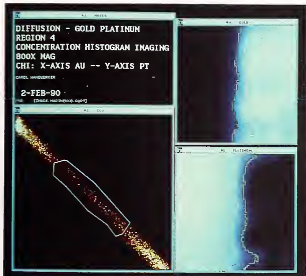
Figure 11. Application of the composition histogram image technique to a diffusion zone between gold and platinum. The compositional range outlined in white in the CHI selects the pixels outlined in white in the original compositional maps, showing the location of the diffusion zone. Image width = 125 micrometers (sample courtesy C. Handwerker, NIST; images courtesy R. Marinenko and D. Bright, NIST).
