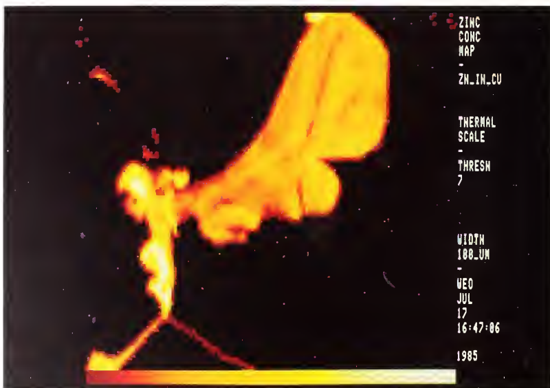
Figure 6(c). Pseudocolor scale constructed from the thermal scale, the sequence of black body colors; the color scale = 0-10 weight percent. Image width = 100 micrometers (specimen courtesy D. Butrymowicz, MSEL, NIST).
