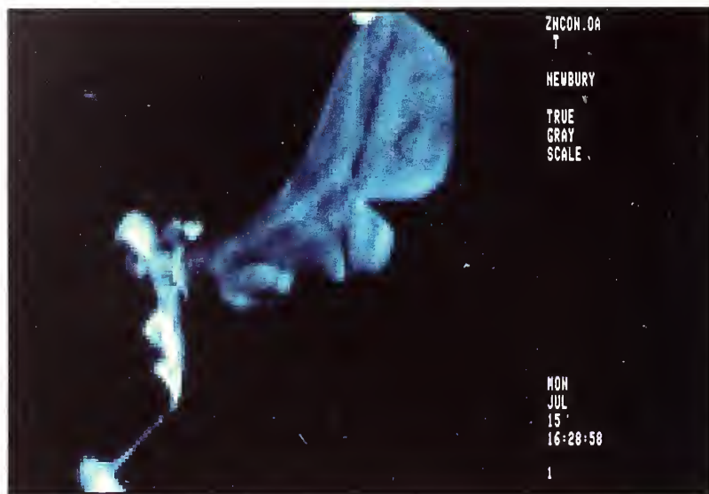
Figures 6(a) through 6(c). Compositional maps of zinc at the grain boundaries of polycrystalline copper as a result of diffusion-induced grain boundary migration. Figure 6(a). Gray-scale presentation (0-10 weight percent corresponds to the range from black to white).
