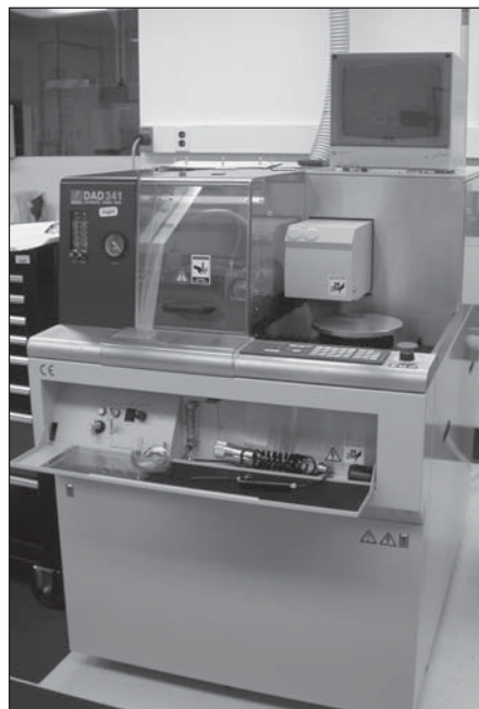
Automatic 8" wafer dicing saw.
