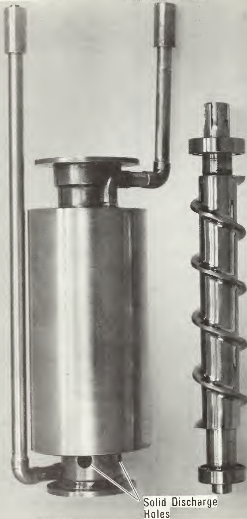
Figure 2. Partially disassembled auger unit.
