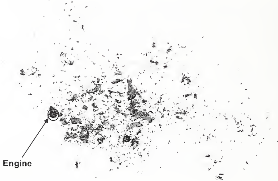
(b) Aircraft debris field (time=0.62 s)
