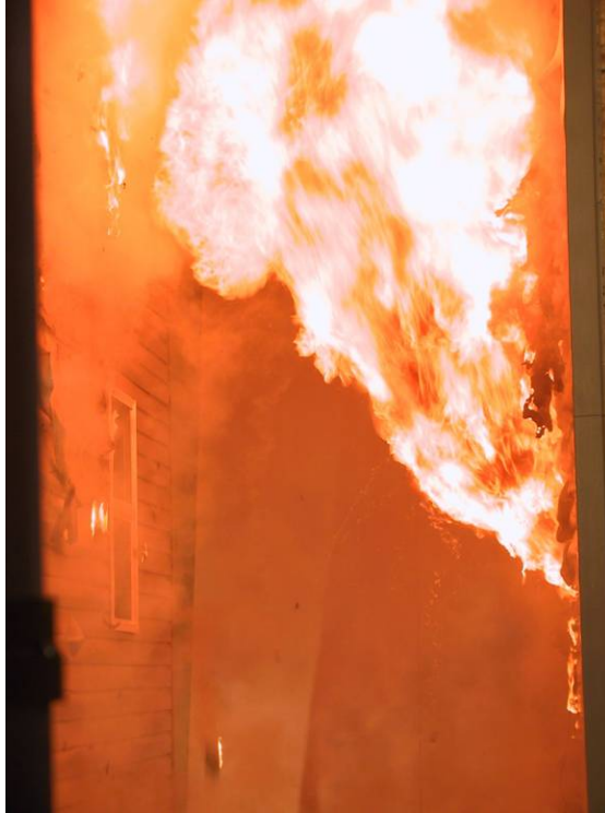
Figure 15. Unrestricted Construction Experiment: Target Wall OSB Ignited 1 min 20 s after Window Failure
