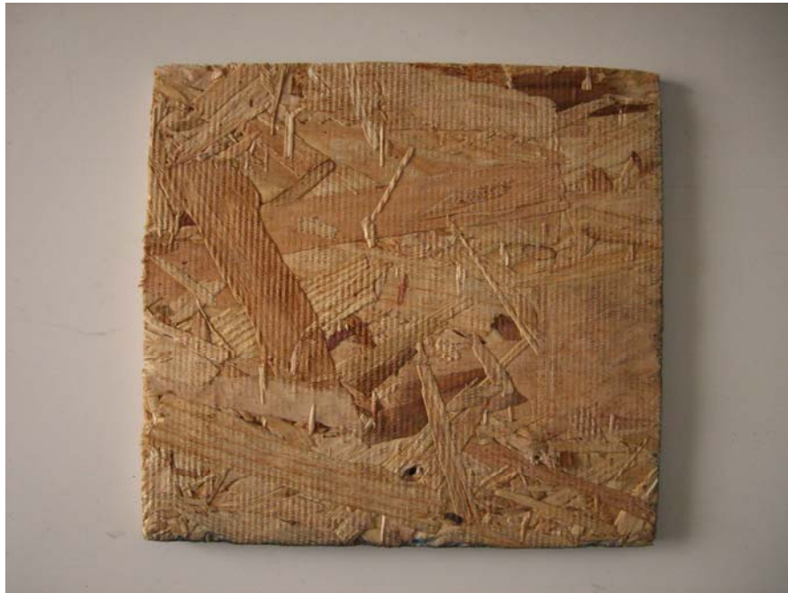
Figure 11: Sample of unburned OSB from Target Wall - Experiment 2
