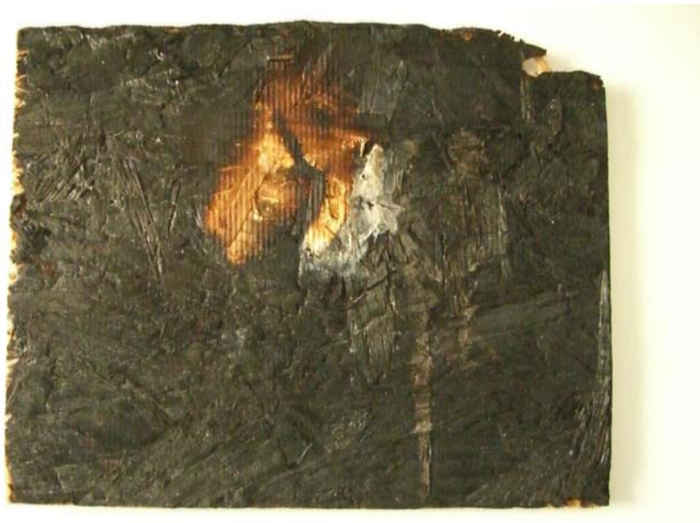
Figure 10: Sample of burned OSB from Target Wall - Experiment 1
