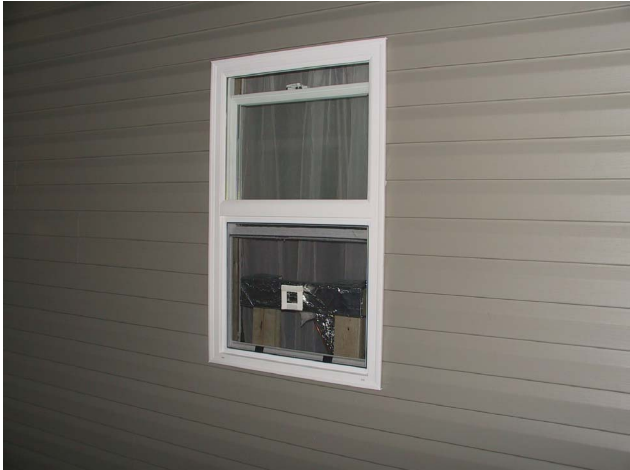
Figure 8: Photograph of flux gauge (FG3) in target wall window looking at structure of fire origin.
