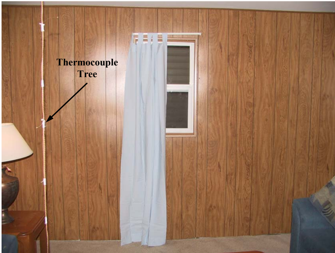
Figure 6. Photograph showing interior of room of origin including wall, window, curtain, some furniture, and a thermocouple tree.
