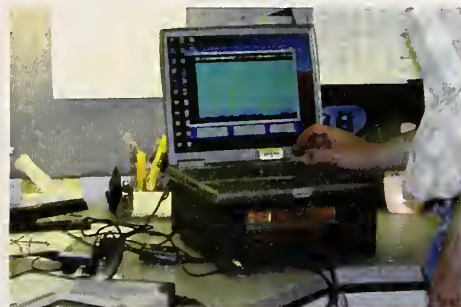
Figure 2.2-1: Illustration of the narrowband received-power measurements. (a) A radio transmitter was carried throughout the building on a continuous path, and the signal strength was recorded by the receiver. (b) The radio transceivers used in the tests were placed in protective cases with additional batteries and modified for continuous transmission. (c) The receiver consisted of a commercially available communications receiver, followed by post-processing steps to determine the received-signal level.
