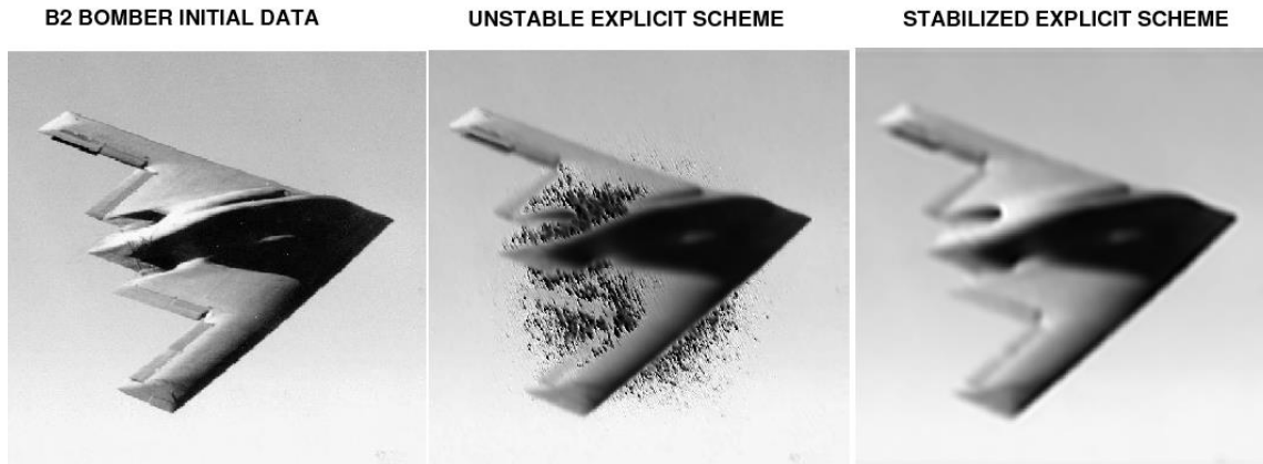
Figure 35. Useful computation of well-posed forward nonlinear parabolic problems on 512 \times 512 mesh, using stabilized explicit scheme with a value of \Delta t that is unstable in the uncompensated pure explicit scheme.
