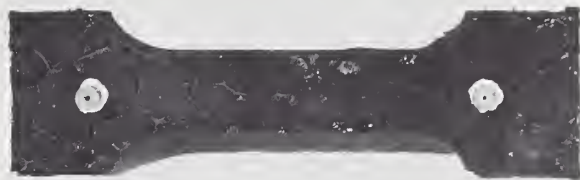
FIGURE 2. A prepared test specimen of a membrane taken from the field after nine years exposure.
