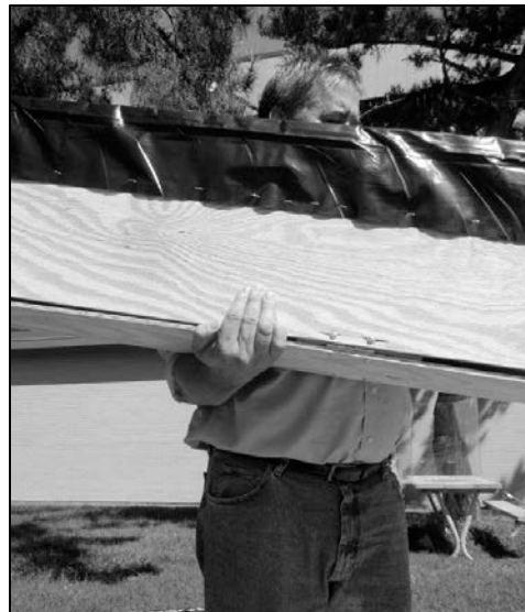
Figure 3-22. How to Cradle the Chute. Cradle the chute on one arm while holding it with one hand and tilting the cradle with the other hand.
