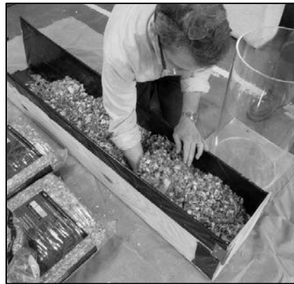
Figure 3-20. First Pour into the Test Measure.
