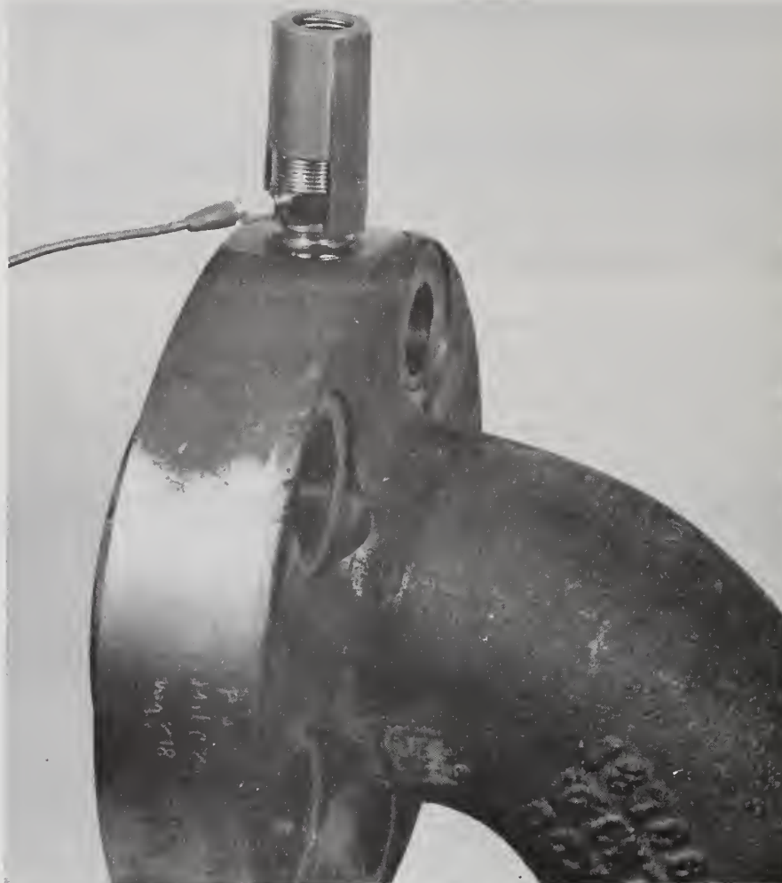
Figure 5 - Transducer Clamped to Mounting Disc
