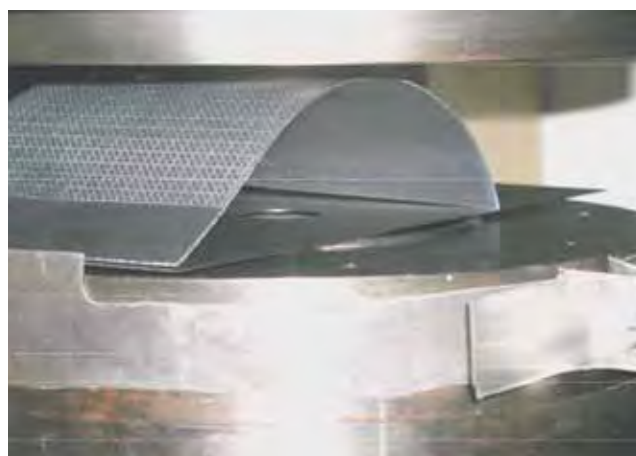
Figure 12: NUMISHEET benchmark sample in the Formability Station being loaded in plane strain.
