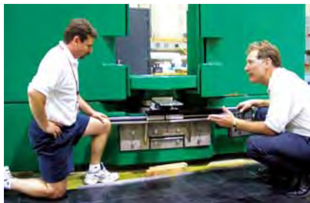
Figure 19: Peter Hundertmark and Timothy Pike examine the ball screw mechanism that will rotate the sample and detector around the green monochromatic beam transport system, which they designed.
