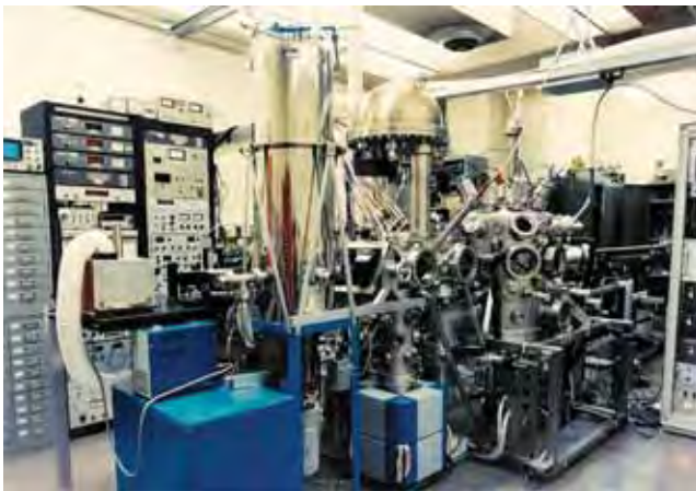
Figure 14: The Magnetic Engineering Research Facility is the world's most elaborately instrumented system for magnetic thin-film deposition and in situ characterization.
