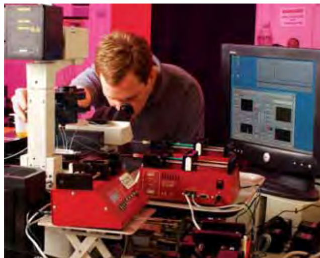
Figure 6: Phillip Stone using microfluidic interfacial tensiometer.
