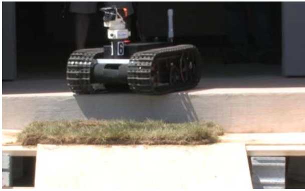
Figure 20. Talon approaches a drop-off to sod.
