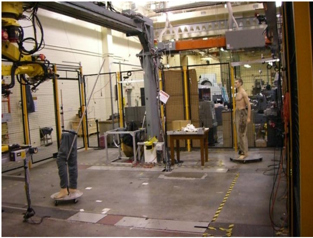
Figure 8. Robot testbed with mannequins moved into places selected randomly by computer.
