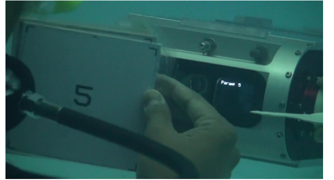
(b) Example of command acknowledgement given on the LED screen of the Aqua robot during field trials.
