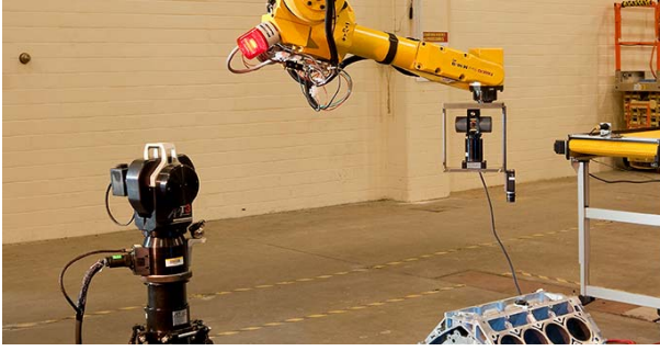
Figure 1. The laser tracker ground truth system (left) and active target attached to an industrial robot arm (right).
