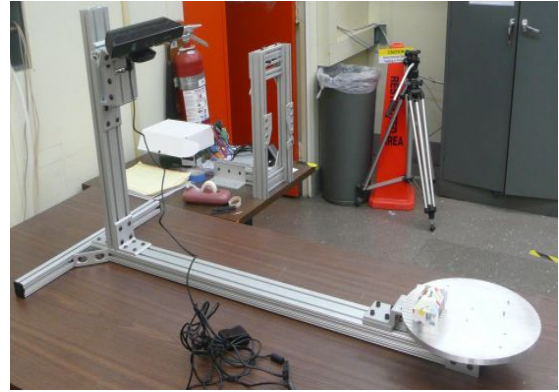
Figure 2. The 6DOF ground truth fixture with an attached sensor and artifact on the rotation plate.
