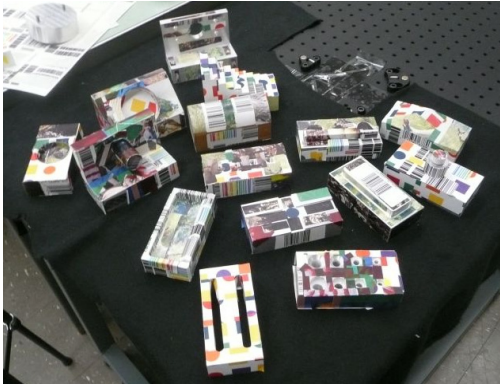
Figure 1. The sixteen machined NIST artifacts used in the 2011 SPC, arranged randomly.
