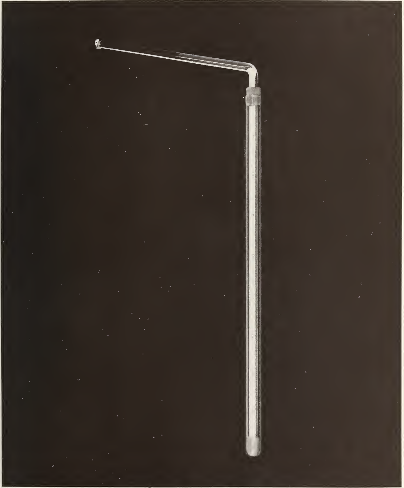
Figure C-8. Ground-temperature probe. C-15
