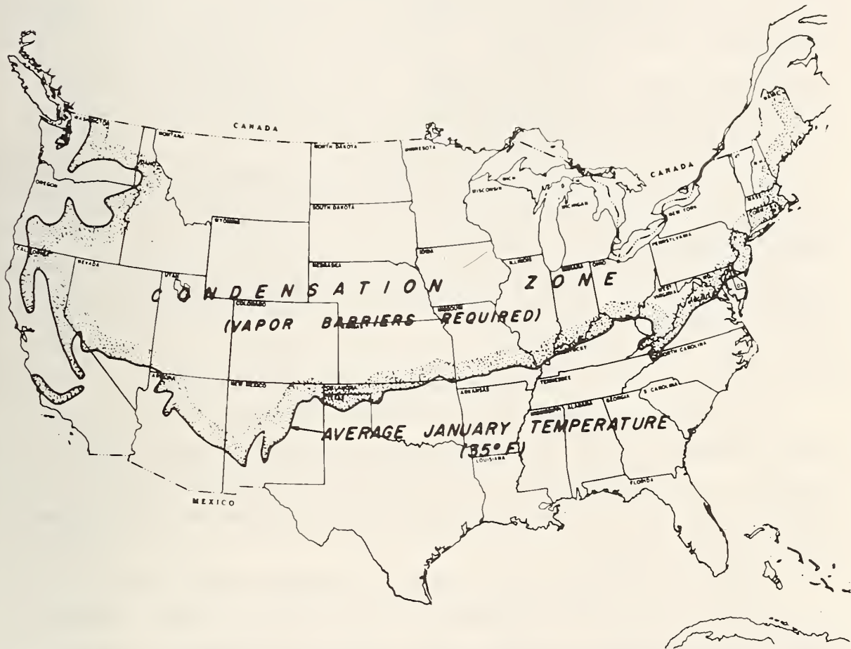
Figure 4-6. Winter condensation problems occur where the average temperature for January is 35° F or lower (taken from "Condensation Problems: Their Prevention and Solution," by L. A. Anderson, U.S.D.A. Forest Service Research Paper FPL 132, Forest Products Laboratory, Madison, Wisconsin, 1972).
