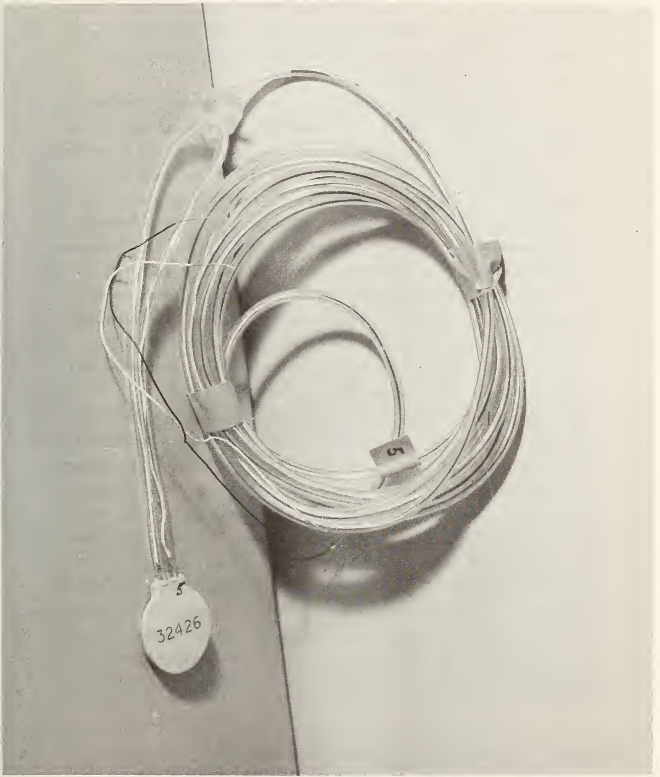
Figure C-11. Heat-flux meter for heat-loss measurement.
