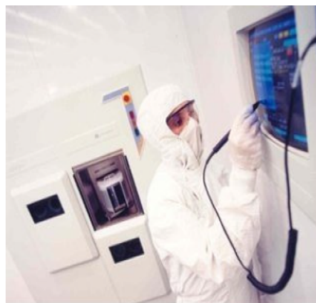
A technician programs a product "Recipe" into an epi reactor.
