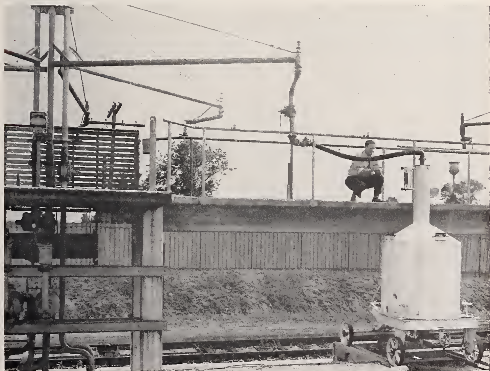
FIGURE 8. Semiportable prover tank, capacity, 500 gallons.
