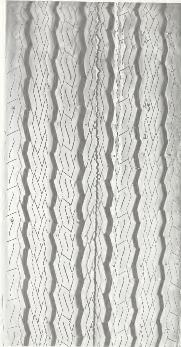
Figure A-2. Characteristic tread element pattern of tire-C (bias-belted rib). The nominal new tread depth for this tire was 13/32 inch. Shore hardness values ranging from 59-62 were observed with the average being 60. The nominal worn tread depth for this tire was 8/32 inch and the Shore hardness values ranged from 61-62 with the average being 61.
