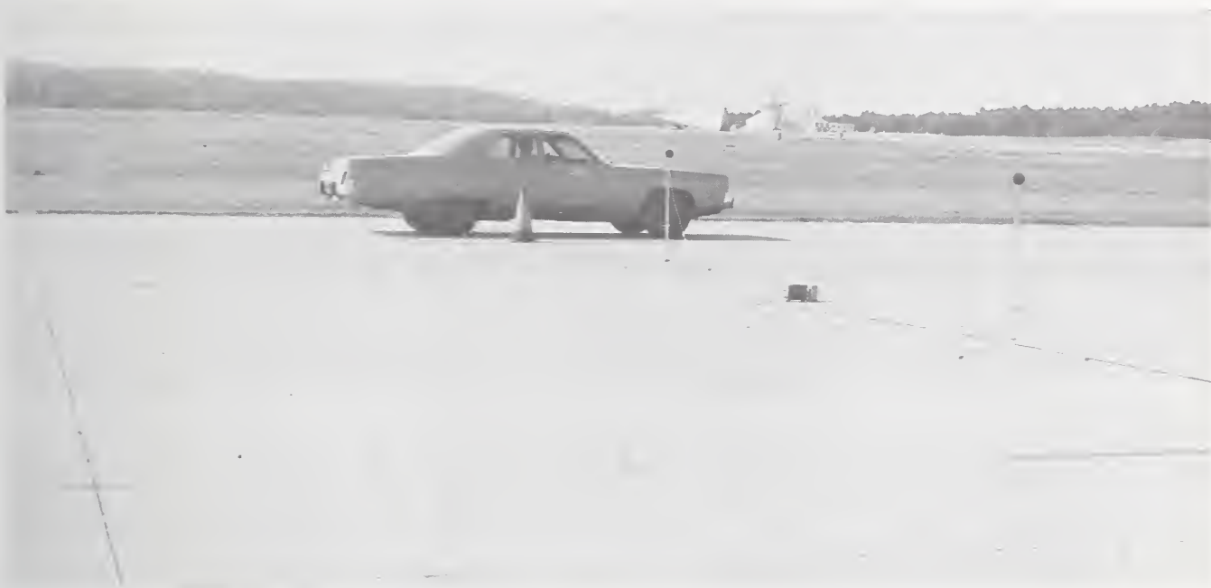
Figure 12. Overall view of the microphone array with the test vehicle (concrete test section, Wallops Station site). The array consisted of two tripod-mounted microphones located at 25 and 50 feet (7.6 and 15.2 m) from the centerline of vehicle travel along a line perpendicular to the vehicle path.
