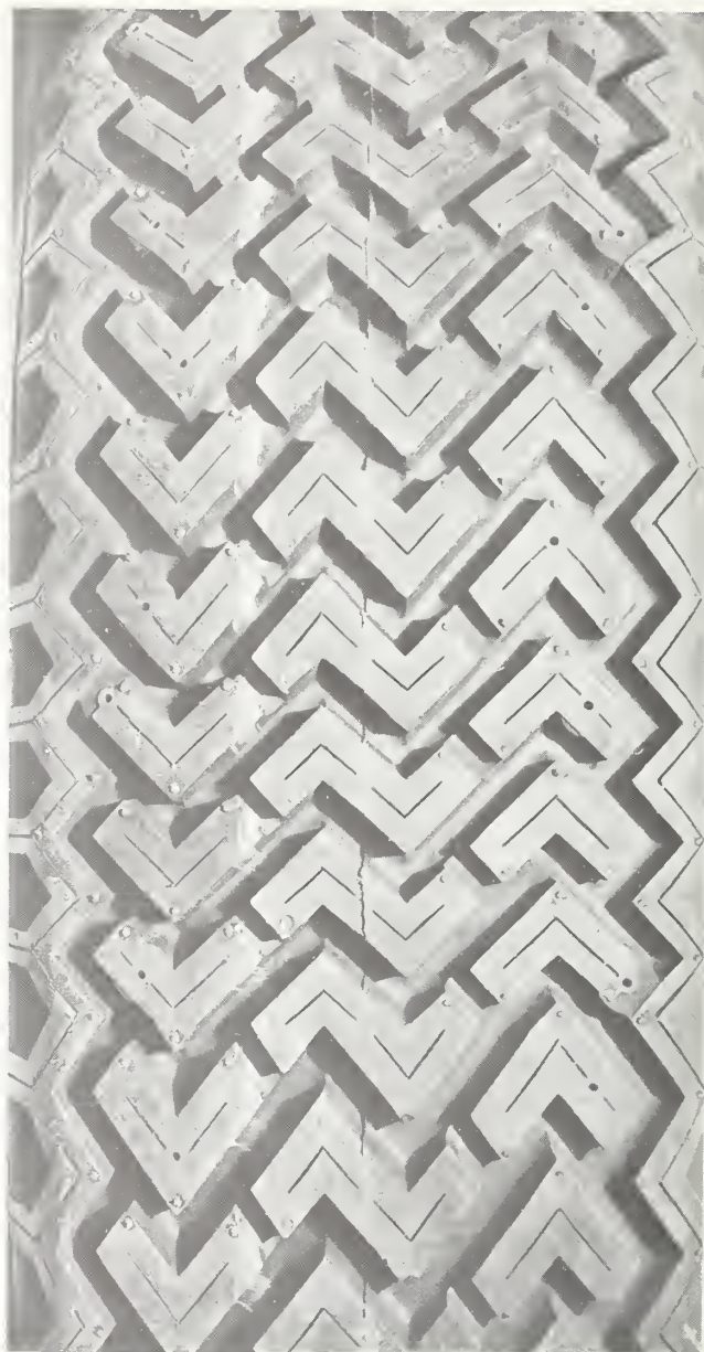
Figure A-4. Characteristic tread element pattern of tire-E (radial snow). The nominal new tread depth for this tire was 14/32 inch. Shore hardness values ranging from 56-60 were observed with the average being 59. The nominal worn tread depth for this tire was 8/32 inch and the Shore hardness values ranged from 58-68 with the average being 60.
