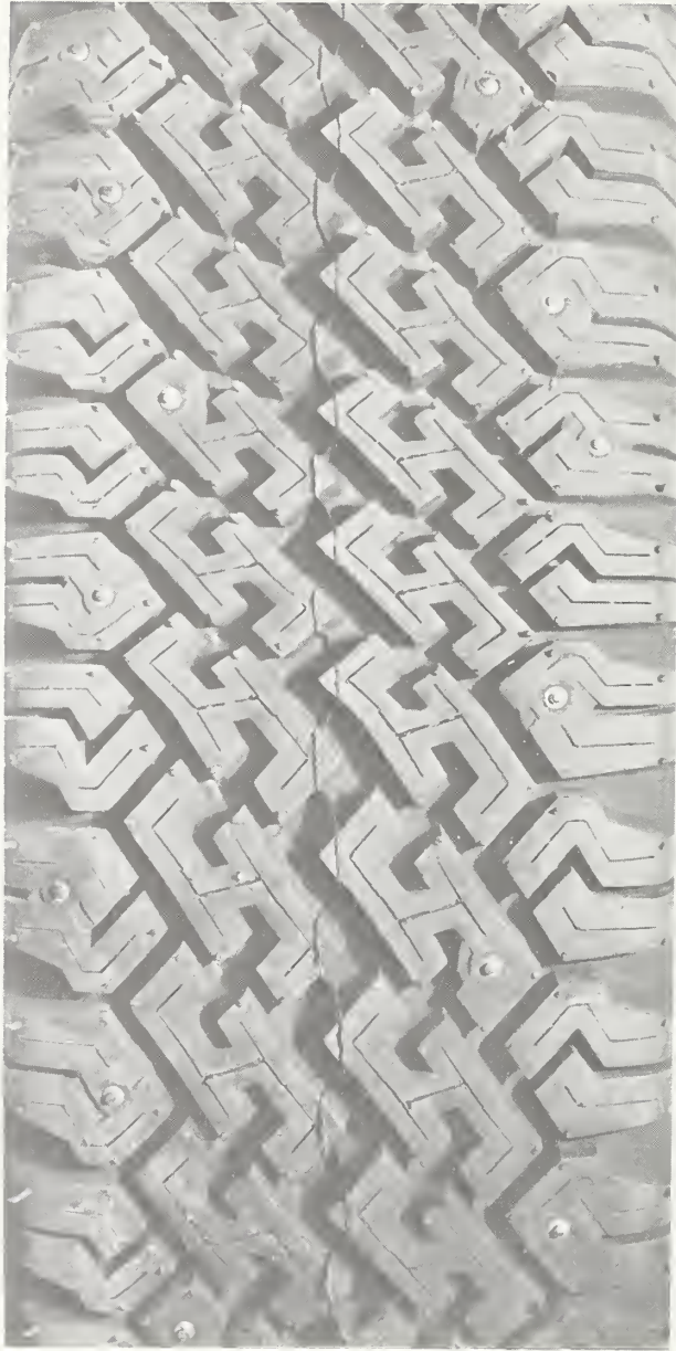
Figure A-6. Characteristic tread element pattern of tire-G (bias-ply studded snow). The nominal new tread depth for this tire was 13/32 inch. Shore hardness values ranging from 55-60 were observed with the average being 58. The nominal worn tread depth for this tire was 6/32 inch and the Shore hardness values ranged from 60-62 with the average being 61.
