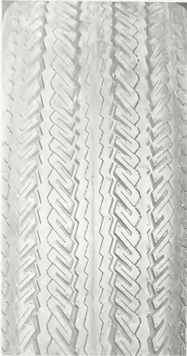
Figure A-3. Characteristic tread element pattern of tire-D (radial rib). The nominal new tread depth for this tire was 11/32 inch. Shore hardness values ranging from 60-65 were observed with the average being 63. The nominal worn tread depth for this tire was 8/32 inch and the Shore hardness values ranged from 60-64 with the average being 62.
