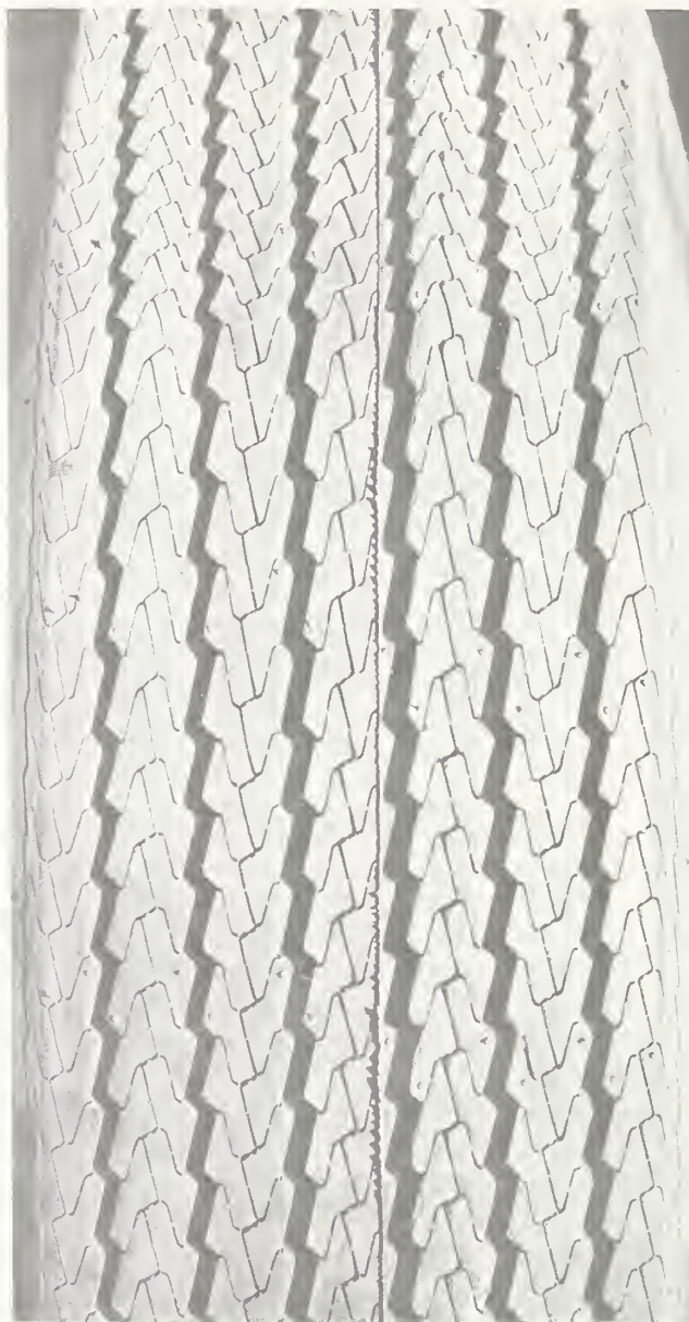
Figure A-1. Characteristic tread element pattern of tire-B (bias-ply rib). The nominal new tread depth for this tire was 12/32 inch. Shore hardness values ranging from 58-61 were observed with the average being 60. The nominal worn tread depth for this tire was 7/32 inch and the Shore hardness values ranged from 60-64 with the average being 62.
