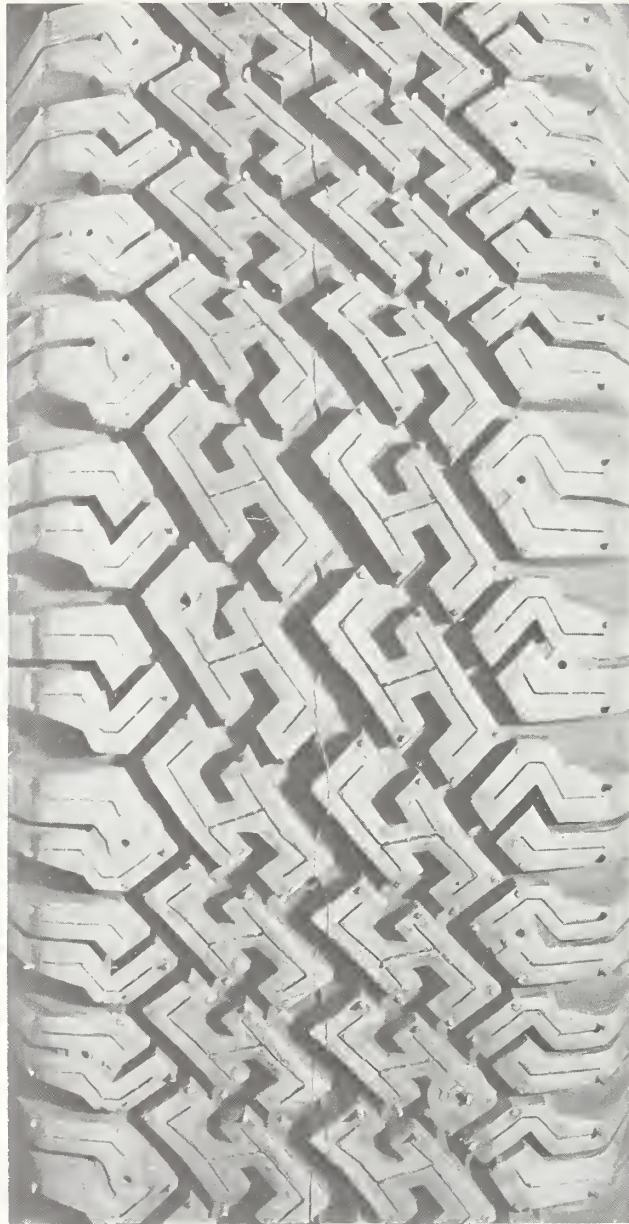
Figure A-5. Characteristic tread element pattern of tire-F (bias-ply snow). The nominal new tread depth for this tire was 13/32 inch. Shore hardness values ranging from 59-61 were observed with the average being 60. The nominal worn tread depth for this tire was 6/32 inch and the Shore hardness values ranged from 59-60 with the average being 60.
