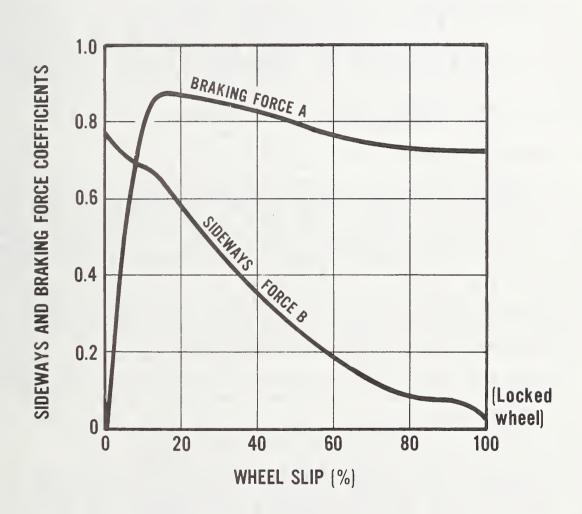
Figure 7. Relationship of wheel slip to braking and controllability.
