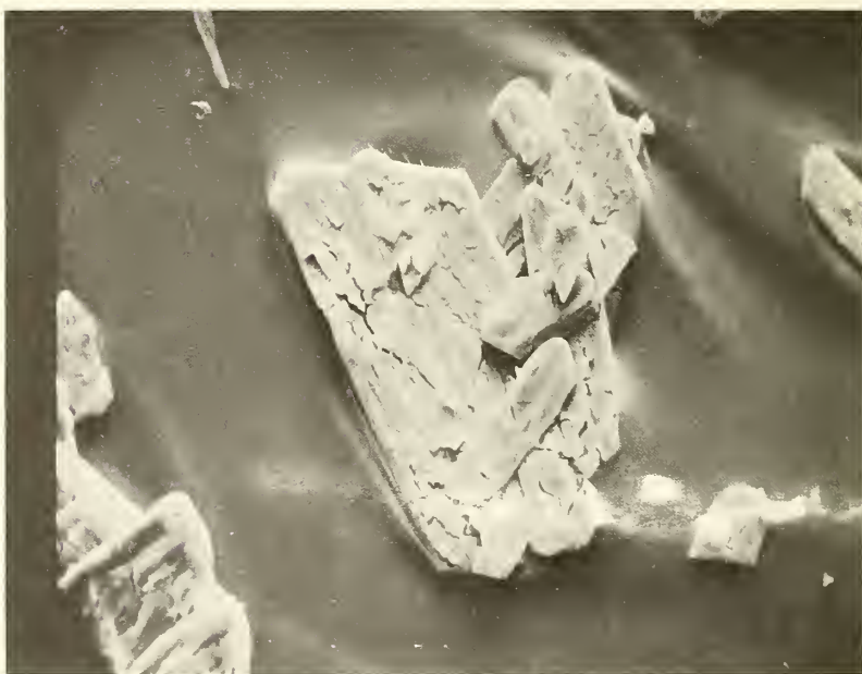
Figure 8 Scanning electron micrograph of plaster of paris, X 2000.
