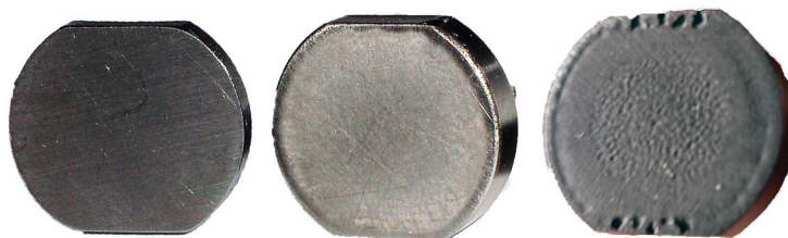
Figure 3. Surface appearance for removable ½” flat tip, ranging from pristine (left), to matted (center), to badly eroded with pitting (right).
