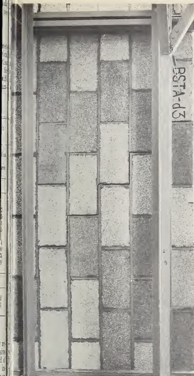
FIGURE 19. Flexural bond failure of concrete masonry wall BS-P3, tested with bed joints parallel to span.
