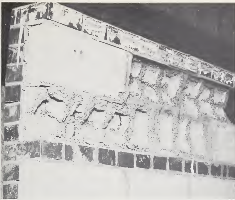
FIGURE 6. Compressive load failure of composite masonry wall
