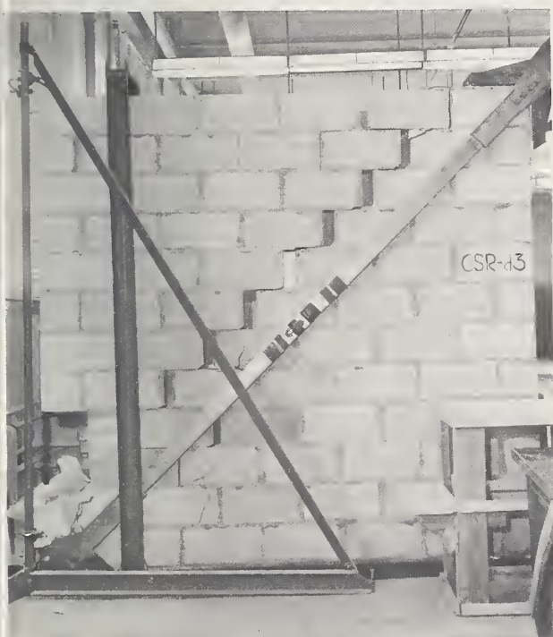
FIGURE 12. Shear failure of concrete masonry wall CS-3.
