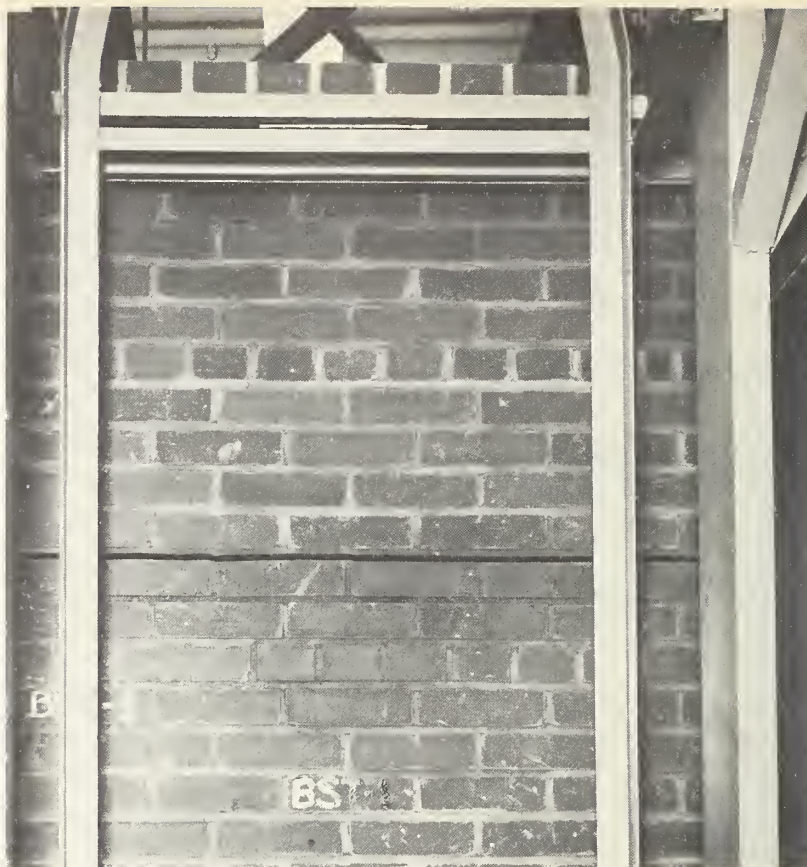
FIGURE 23. Typical flexural bond failure between stretcher courses in brick facing of composite walls.
