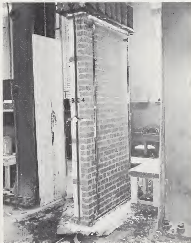
FIGURE 5. Composite masonry wall ready for compressive strength test.
