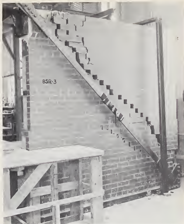
FIGURE 13a. Shear failure in brick facing of composite masonry wall BS-3.
