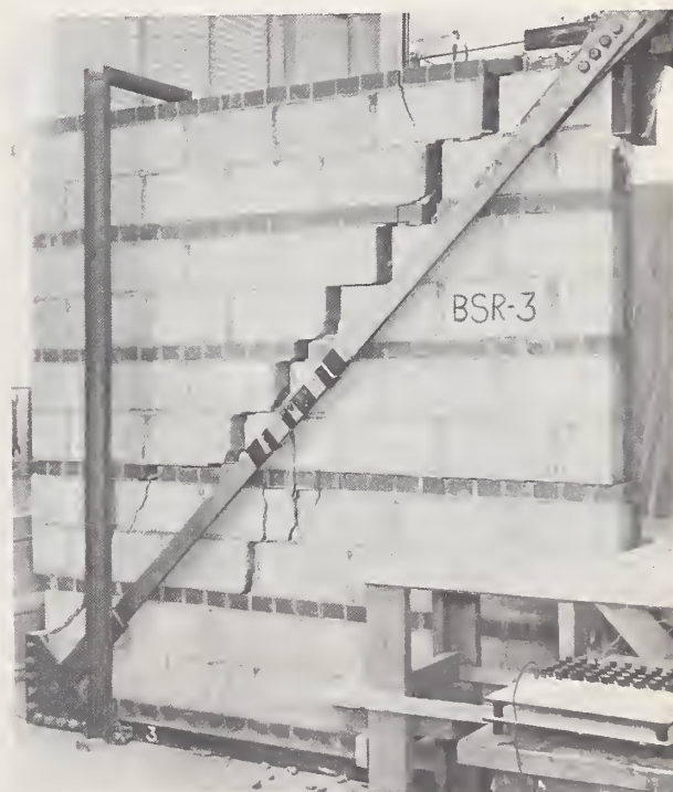
FIGURE 13b. Shear failure in block backing of composite masonry wall BS-3.
