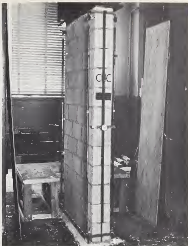
FIGURE 4. Concrete masonry wall ready for compressive strength test.
