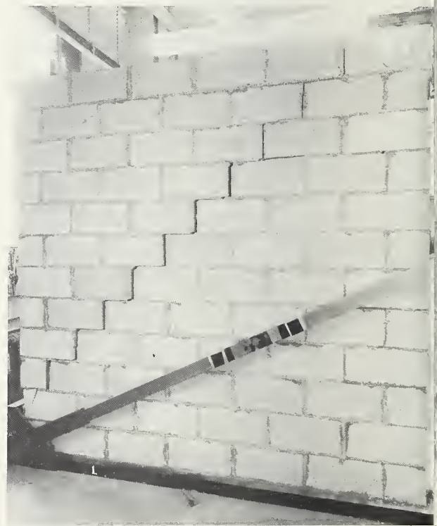
FIGURE 10. Shear failure of concrete masonry wall BN-1.
