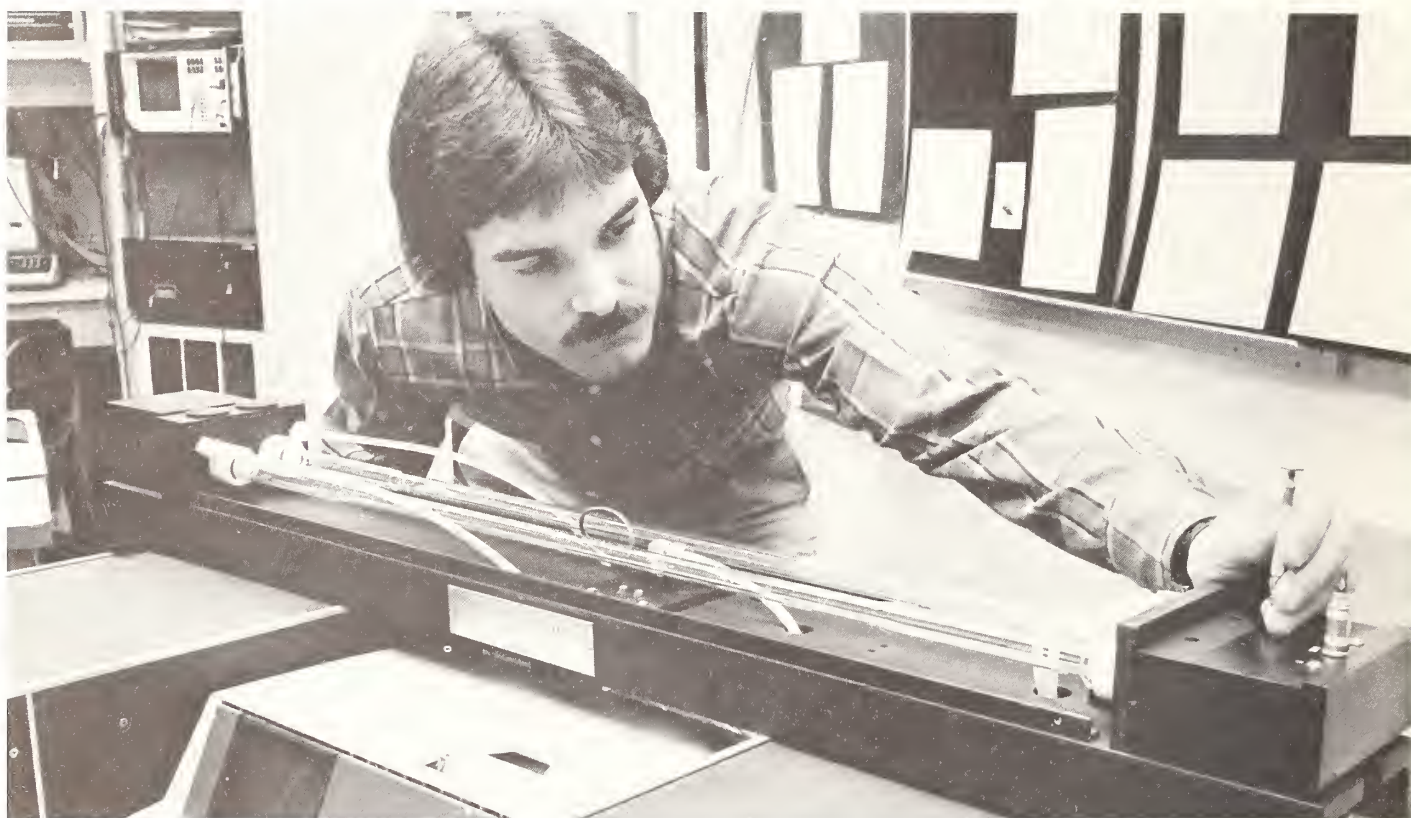
NBS technician Jim Norris adjusts the Bureau's ozone reference photometer which is used as a "definitive" standard for calibrating the reference photometers in EPA regional laboratories.
