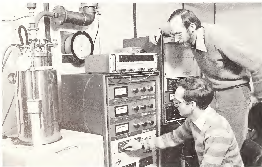
Electrical engineer Bruce Field (sitting) and physicist Marvin Cage use an automated system developed at NBS to monitor the quantum Hall resistance phenomenon against the electrical resistance standard maintained by NBS. The quantum Hall effect may become the basis for a new standard of electrical resistance based on fundamental neutral constants.
