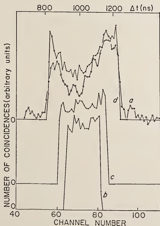
Fig. 3 - CH_4^{++}(\tilde{a}^1E) \rightarrow CH_2^+ + H^+ + H dissociation. Experimental (curve a ) and simulated (curves b , c , d ) PIPICO spectra at E_{exc} = 42 eV. (see text for details)
