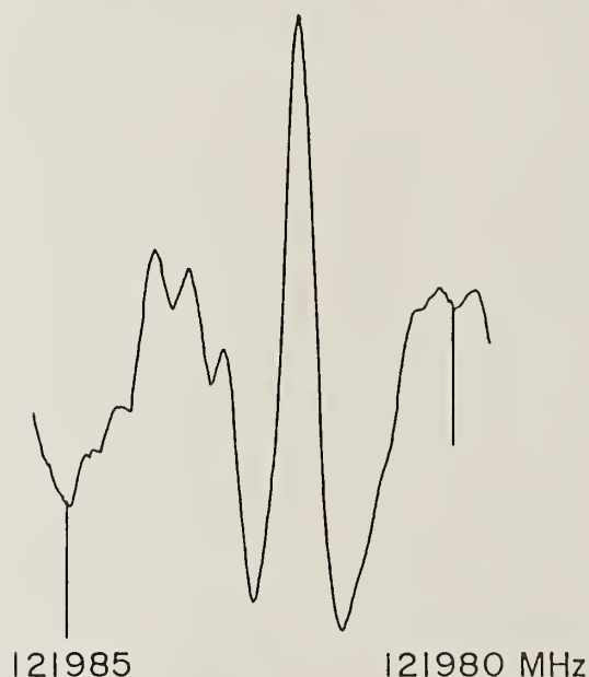
Fig. 1. The J = 11 - 10 transition of ^{18}\text{O}^{13}\text{C}^{34}\text{S} in natural abundance (0.96 ppm) observed by an integration of 50 s with the 3.5 m free space cell and source modulation.
