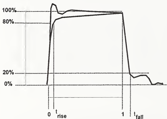
Fig 2. Schematic of 1 nsec VCSEL pulse showing characteristic features.
