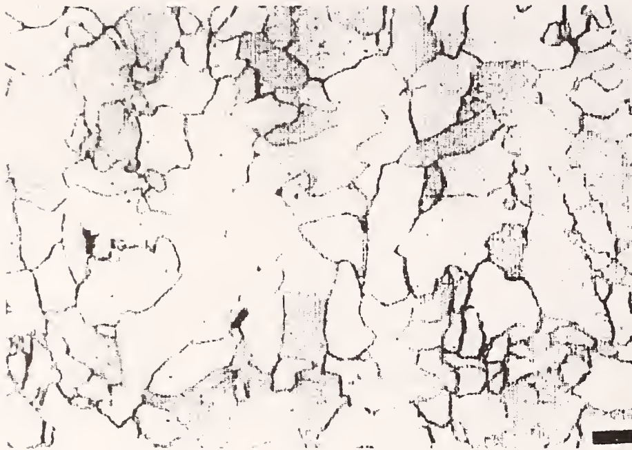
Figure 9. Typical microstructure for HSLA-V, 350 MPa grade. Bar in picture represents 10 \times 10^{-3} mm.
