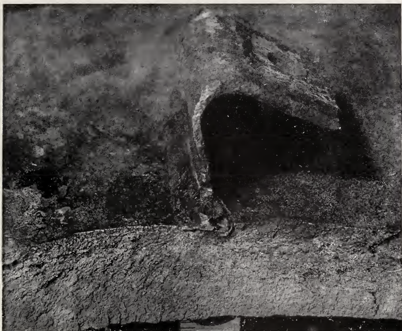
FIGURE 9.6. Source of fracture shown in figure 9.5 at arc craters in weld of small clip to deck.
