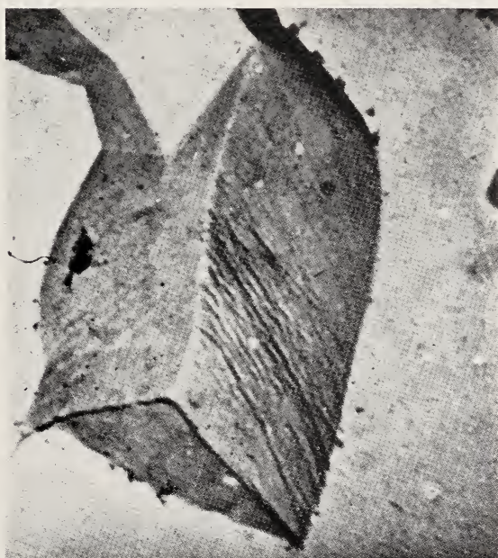
FIGURE 1.10. Slip zones in aluminum at 500^{\circ}\text{C} , \times 25,000 . (A. F. Brown)
