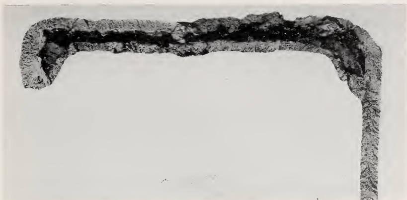
FIGURE 9.2. Fracture source in defective weld of bulwark cap rail, \times 2/3 .
