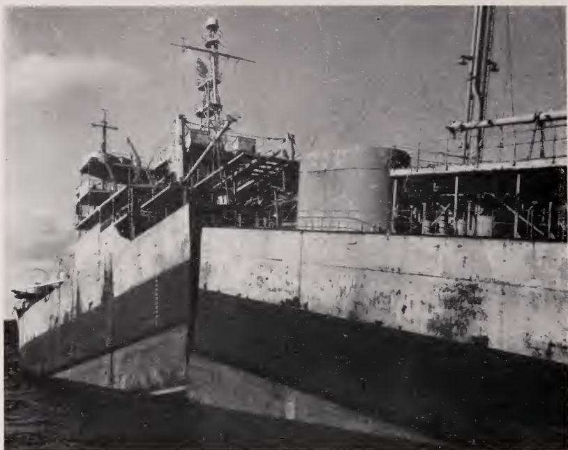
FIGURE 9.5 Tanker that broke in two at dock.
