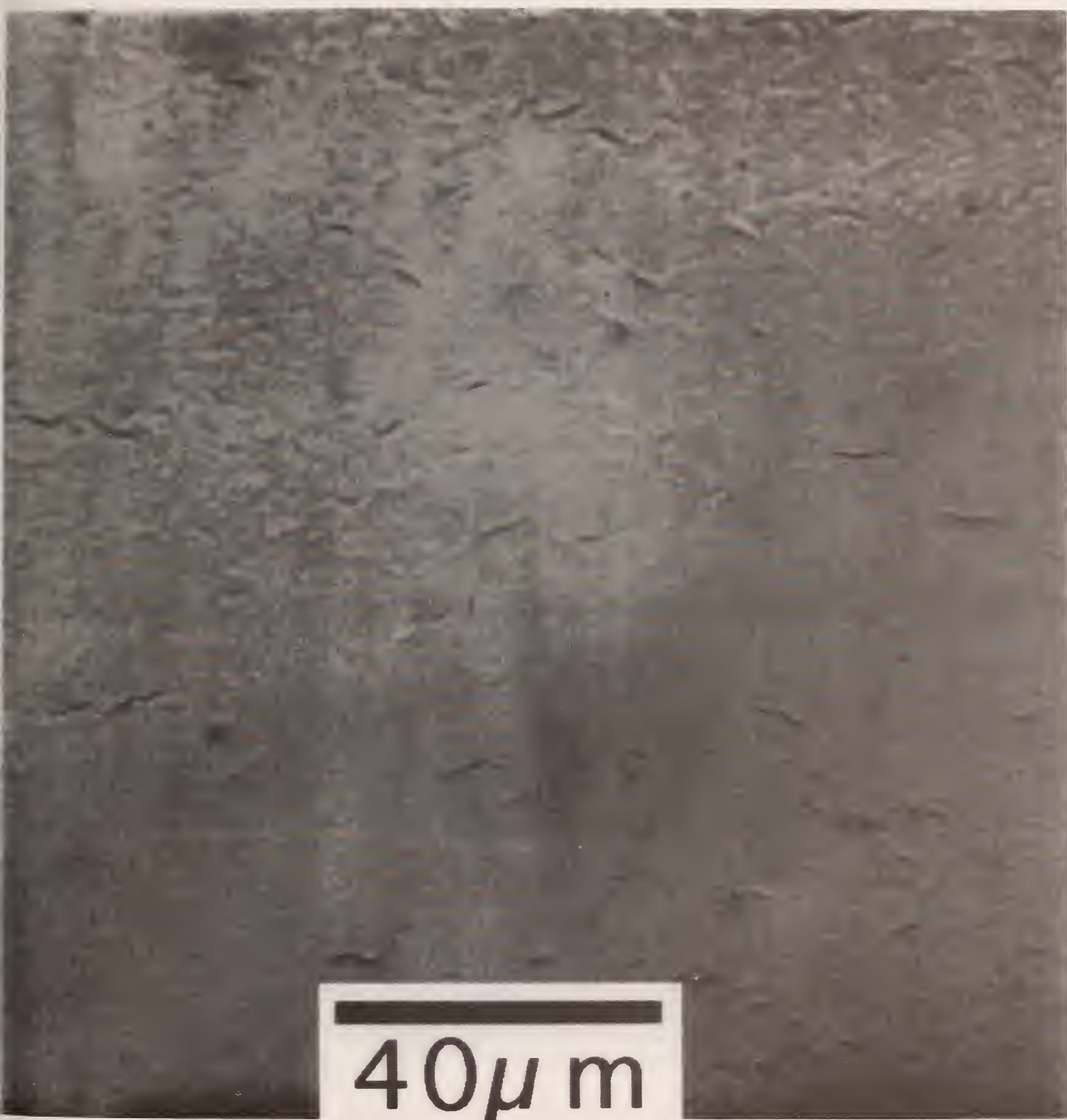
Figure 8. Optical micrograph of the surface of a Ti-coated Cu specimen after fatigue.
