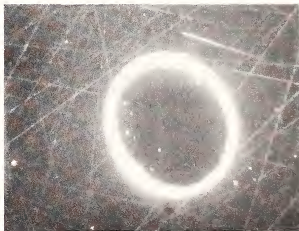
Figure 11 : 'Laser annealed' damage spots on germanium, 10.6 \mu\text{m} (X400)
