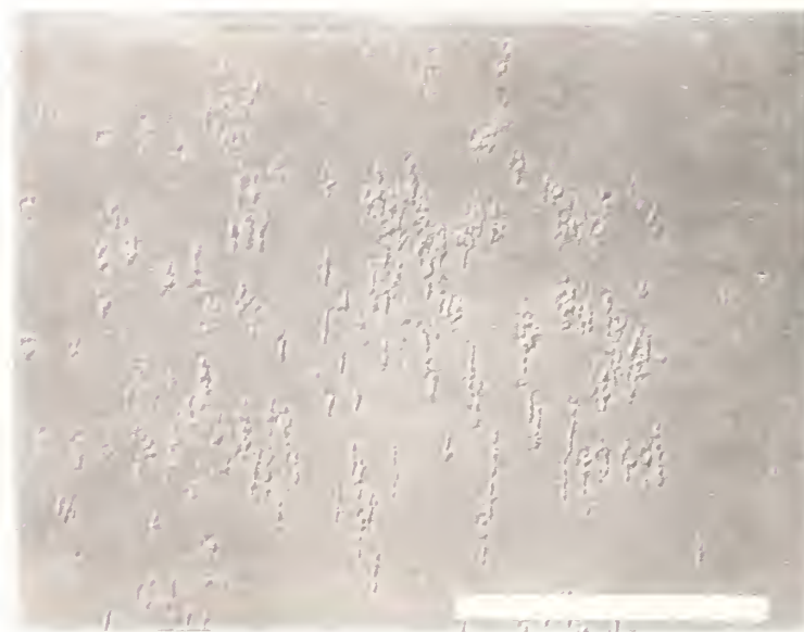
c. Six pulses, 1.12 \text{ J/cm}^2 average fluence, charge emission occurred for the last three pulses. Bar is 50 \text{ }\mu\text{m} .
