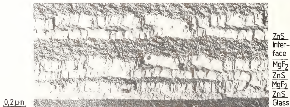
Figure 10. TEM-micrograph of the Pt/C-replica of a \text{ZnS}/\text{MgF}_2 multilayer cross-section, showing nearly amorphous microstructure for the \text{ZnS} layer next to the substrate, whereas the further \text{ZnS} layers exhibit a columnar microstructure.
