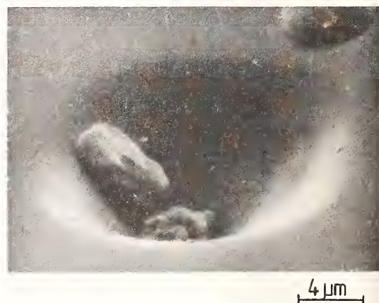
Figure 6. Holes in optical coatings caused by separating nodules (SEM-micrographs) a. nodule popping out as a whole b. secondary nodule growth in a hole
