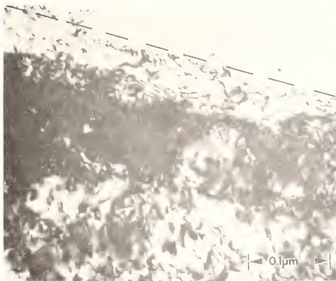
Figure 2. Bright field micrograph of the transverse section of the -5 deg rake surface. The dashed line is the boundary between the sample (lower) and the Cu electroplate (above).
