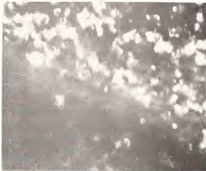
Figure 7. Dark field image of one of the \text{Cu}_2\text{O} spots in the transmission electron diffraction pattern showing the distribution of the oxide. The area is the same as figure 6.
