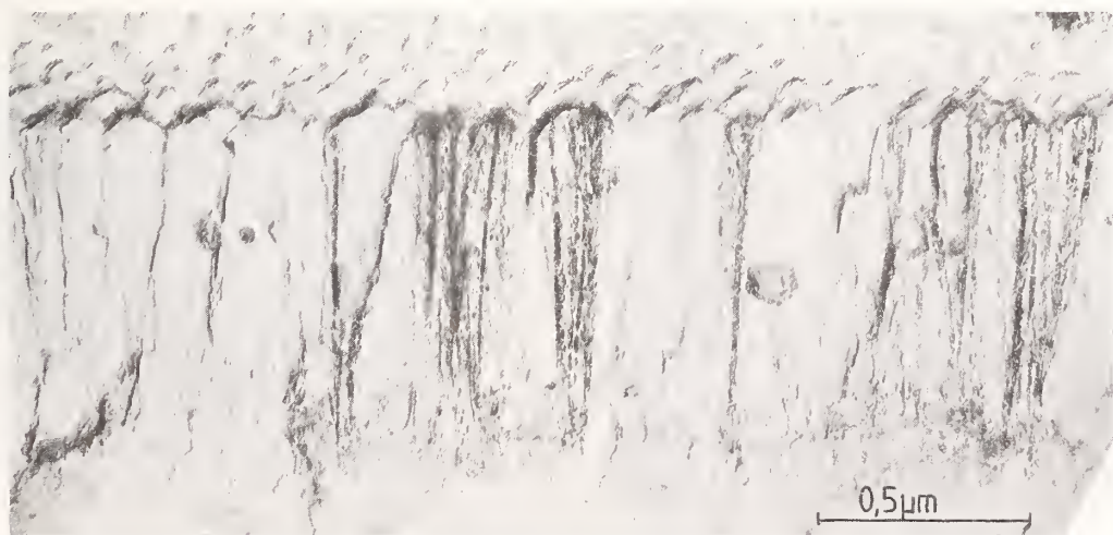
Figure 3. Fibrous substructures in \text{TiO}_2 thin films, disclosed by incomplete dissolution of actual film substance remaining on the carbon replica.
