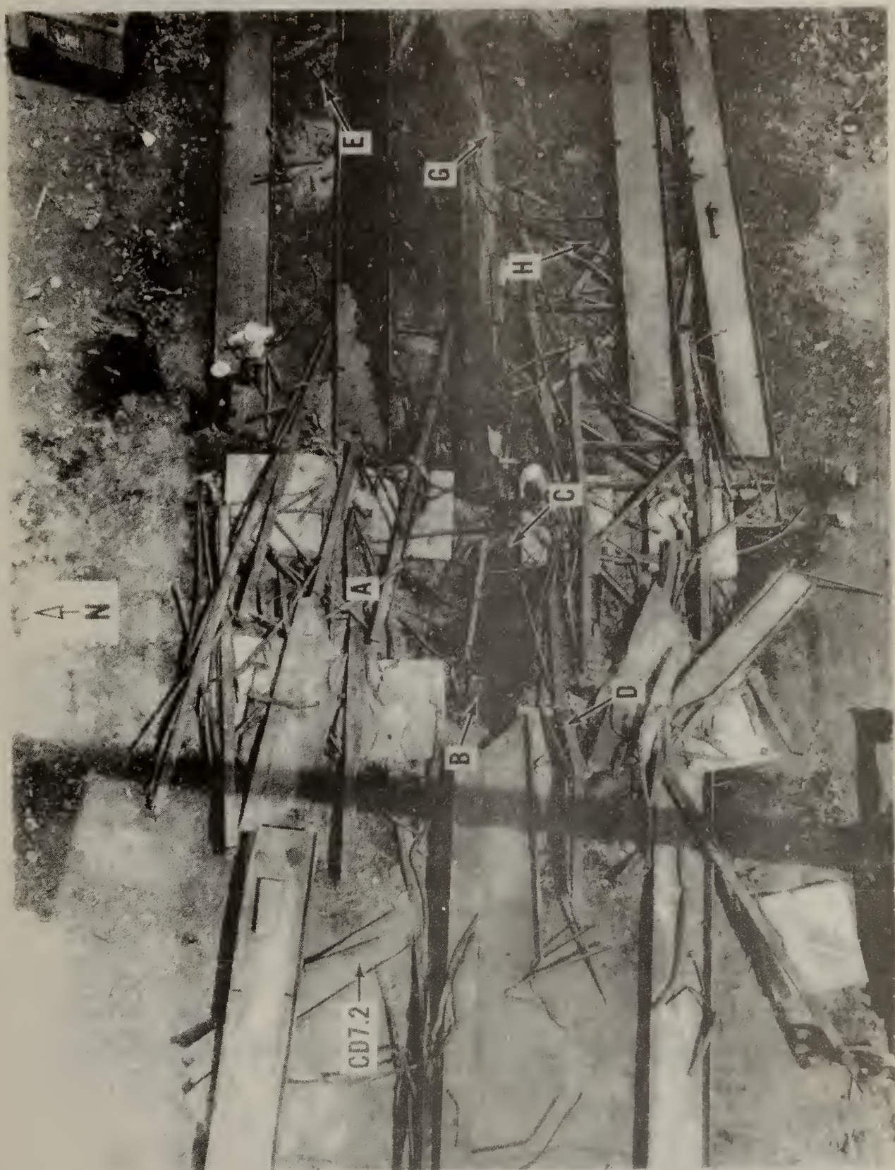
Figure 3.22 Location of tops of U-heads belonging to towers at 407.2
