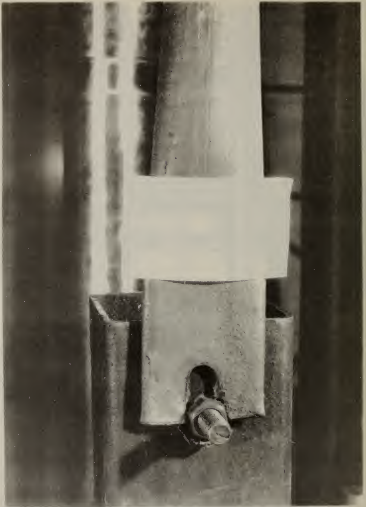
Figure 4.35 Tearing failure at bolt connection of brace #5
