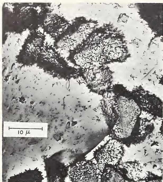
FIGURE 5. Cement paste hydrated 1 hr.
