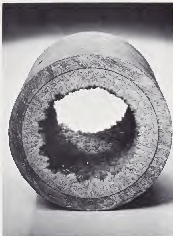
FIGURE 2. Crystalline calcium sulfate deposit in an asbestos cement pipe.
