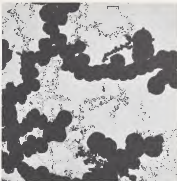
FIGURE 1. Calcium hydroxide chains precipitated from solution in the presence of carbon dioxide contamination.
