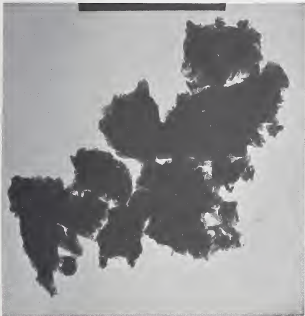
FIGURE 15. Representative aggregates from lightly ground hydrated Type I cement paste. w/c=0.65; age=5½ yr.
