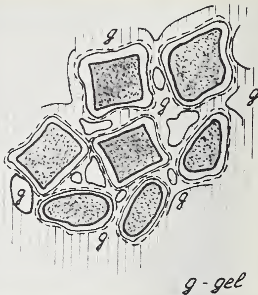
FIGURE 7. Scheme of hardening cement structure.
