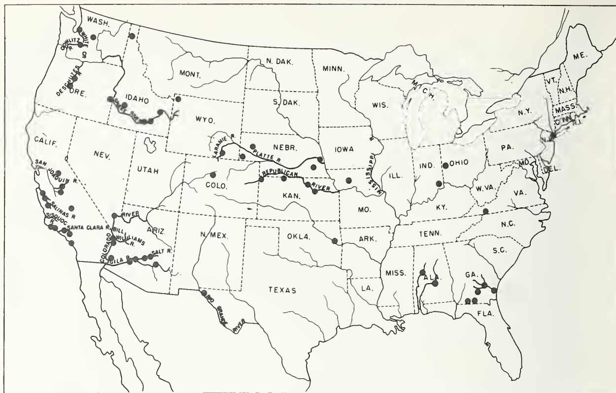
FIGURE 3. Location of structures in the United States known to be affected by, and rivers known to carry, deleteriously reactive aggregate [15].
