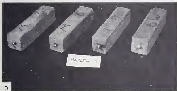
FIGURE 1. Portland cement mortar prisms of granitic aggregate maintained in sea water.
