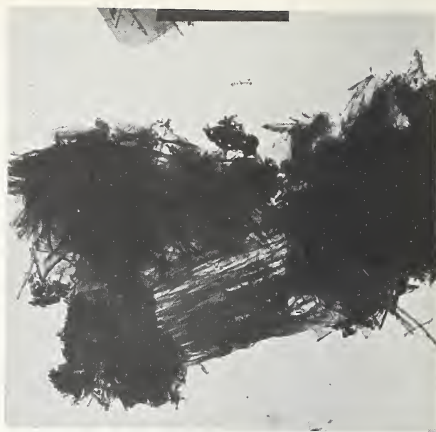
FIGURE 20. Representative fiber bundles from a paste prepared from the 8,000-cm 2 /g fraction of a Type I cement.
