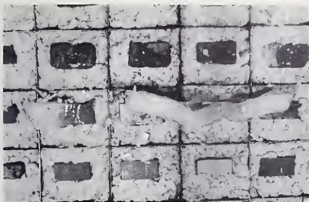
FIGURE 9. Ice lenses formed on clay bricks during slow one-dimensional cooling.
