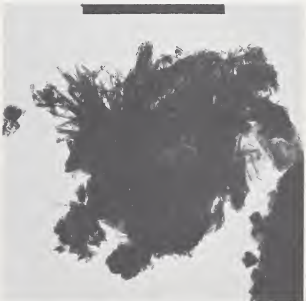
FIGURE 18. Representative gel aggregate from Type III cement paste. w/c=0.6; age=7½ yr.
