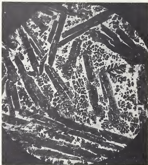
FIGURE 3. Microstructure of granulated clinker. Reflected light. Magnification \times 440 .
