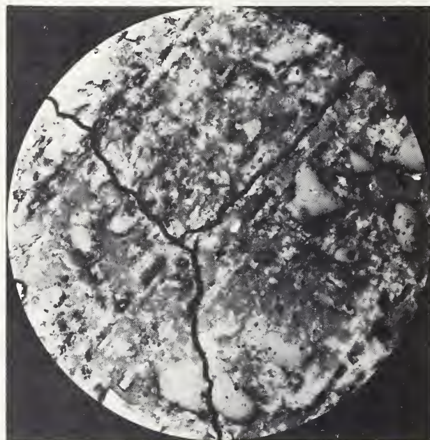
FIGURE 1. Photomicrograph showing unhydrated cement particles.
