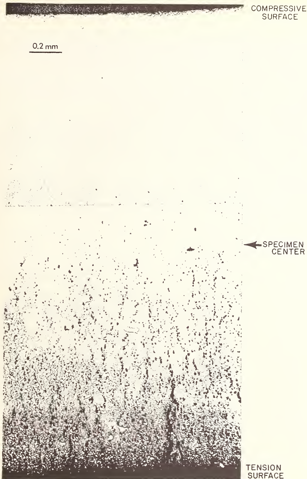
Figure 6. Cavity formation within the cross-section of a siliconized silicon carbide flexure specimen which has been tested at 1300°C and an initial applied stress of 300 MPa [41]. Note that cavity formation on the tensile side of the specimen has proceeded to beyond the original neutral axis of the specimen, indicating a shift in the neutral axis.
