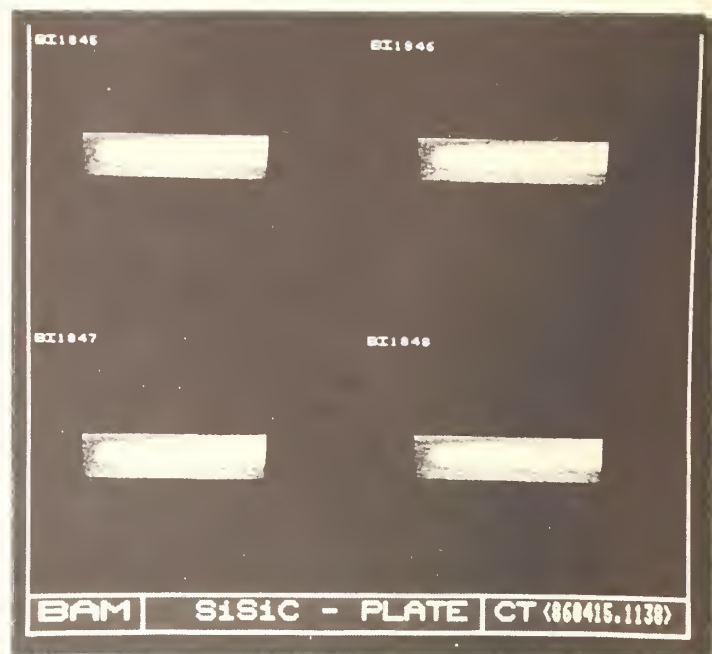
Fig. 2: Four tomograms of a Si impregnated Silicon plate
