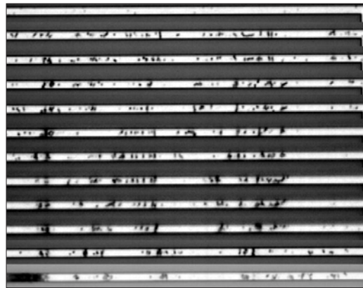
Figure 11. Time-lapse sequence showing rapid voiding (dark spots) in an a. c. test of a damascene copper line in \text{SiO}_2 dielectric. Line dimensions, 3 x 0.5 \mu\text{m} ; peak current density, 16 \text{A}/\text{cm}^2 ; lifetime, 1946 s; temperature range, 403 ^\circ\text{C} .
