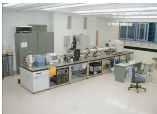
Figure 2. The world's first laboratory scale CD-SAXS prototype constructed on the NIST campus. Shown is the rotating anode molybdenum source (left side) used to generate high energy X-rays for transmission measurements on samples measured at varying angles of incidence on a 2-dimensional detector (back right).
