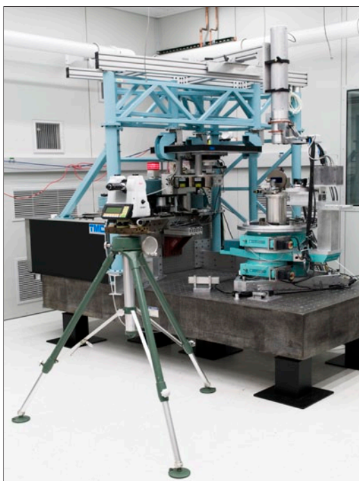
Figure 3. Ceramics Division Parallel Beam Diffractometer (CDPBD) located in the Advanced Measurement Laboratory at NIST seen during alignment of the new spherical air bearing under the goniometers (bottom of green goniometer stack). The X-ray source (near red light in center) is collimated through a monochromator (center, hanging from superstructure) and is diffracted/reflected by a section of a wafer (right) into an analyzer crystal and detector (right). Sample and Detector rotation axes must be coplanar with the incident and diffracted/reflected X-rays. This requires external optical alignment methods using autocollimation, e.g., by a Leika digital theodolite (front, left).
