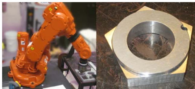
Figure 7: Aluminum pentagonal puzzle insert (right) to be assembled by the ABB IRB-140 open-chain manipulator (left).
