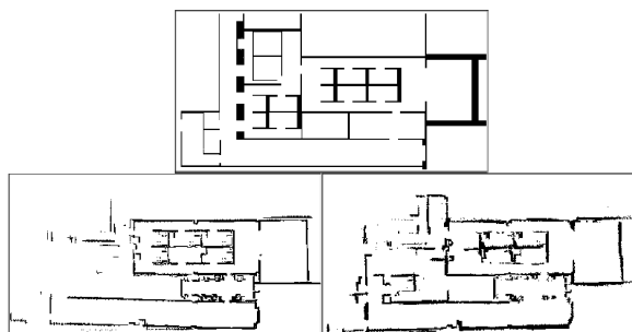
Figure 4: Example for the Metric Quality evaluation, where the upper map is ground truth and the lower-left and lower-right maps are different robot-generated maps.
