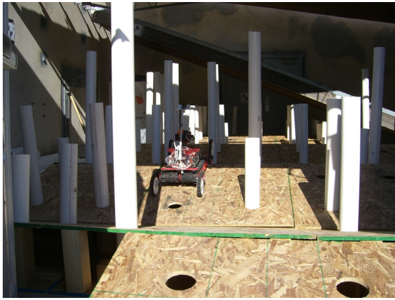
Figure 7: Tube maze test method which tests the mapping ability of US&R robots in an environment littered with occlusions.
