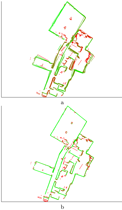
Figure 6: Evaluation of two maps of the data set 'Freiburg082'. a) Quality of map \mathcal{M} = 0.2769 . b) \mathcal{M} = 0.4355 . Colors: level of green (vs red) shows confidence: The greener, the more confident, the more red, the worse. The higher regional confidence in (b) leads to the better total confidence value.
