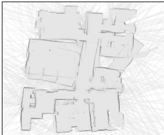
Figure 13 : map built by DP SLAM on real world acquisition “Arcueil laboratory n°1”
