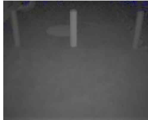
Figure 6: Flash LIDAR Intensity Image of 3 Cylinders in front of the AGV
