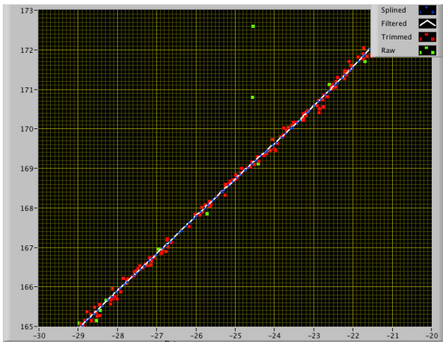
Figure 3. Green is the raw data. Red is the trimmed data. White is filtered data. Blue is the interpolation data
